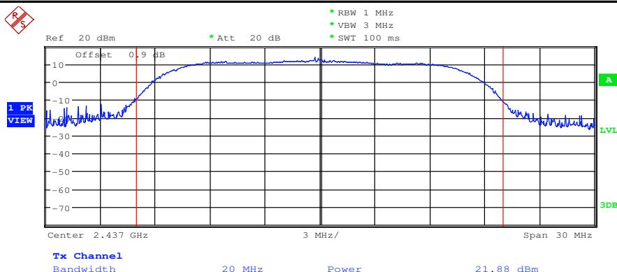
**Maximum peak conducted output power\_11G\_2462\_Ant1**
