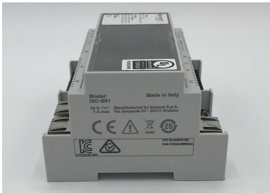
Figure 2: Labels on the product; there are not any difference in the positioning of labels among ISC-B01, ISC-02 and ISC-03
