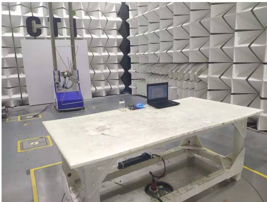
Radiated spurious emission Test Setup-1(Below 1GHz)
