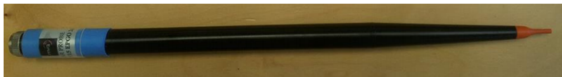
Figure 1 – MVG COMOSAR Dosimetric E field Dipole
