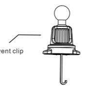
2. After get the air vent clip from the package, align the position of the mounting nut and rotate the nut to clamp the air vent clip
