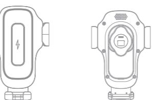
4. After power on, clamp arm automatically open, when the mobile phone put on, clamp arm automatically clamping mobile phone, into the state of wireless charging. The light is now blue. If you want to remove the phone, please touch the sensor switch, arm clamps open, remove the phone.
