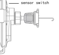
3. Install the assembled wireless charging bracket in the air-conditioning outlet of the car and connect the USB data cable. At this time, the indicator light is blue light breathing (standby)
