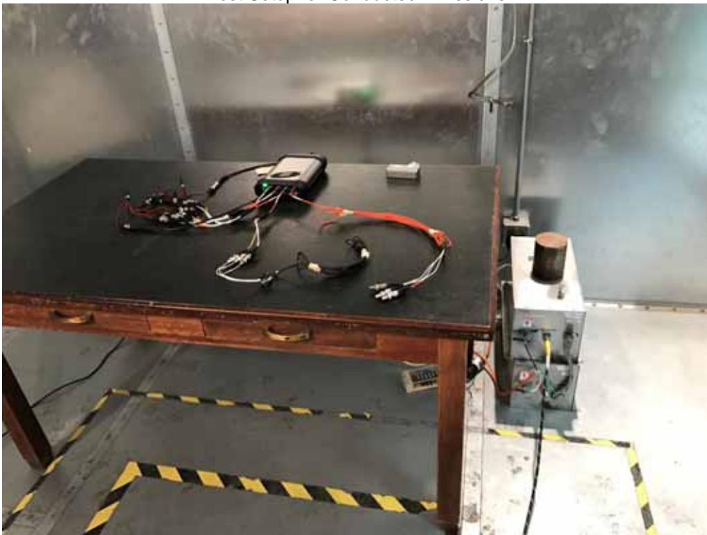
Test Setup for Conducted Emissions
