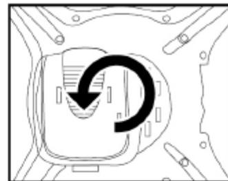
**2.Aiming the camera at the interface on the main body and rotating the camera in anti-clockwise direction to make it screwed.**
