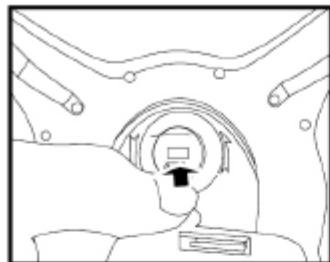
**1.Insert the camera's connector wire into the interface on the main body.**
