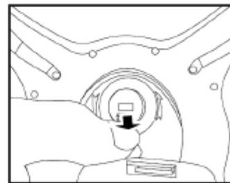
**2.Then taking out the camera upward and pulling out the connector**
