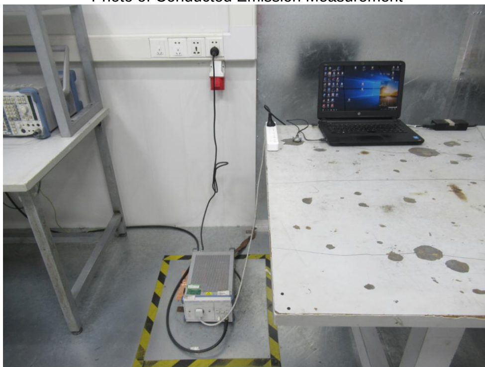
FCC ID: 2ANN4-AFM201T Photo of Conducted Emission Measurement
