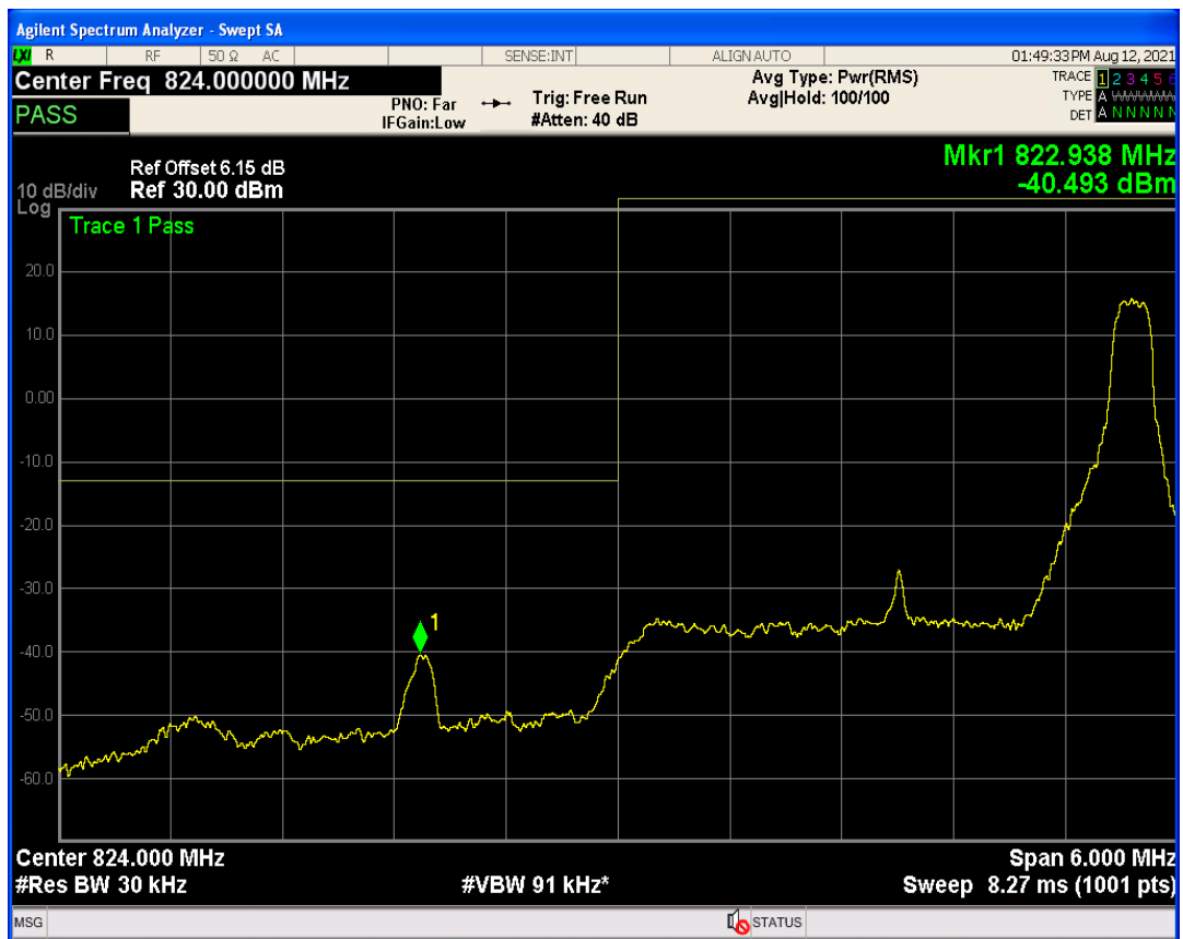
Band5 QPSK BW=3MHz Channel=20635 RB Size=1 Position=#0
