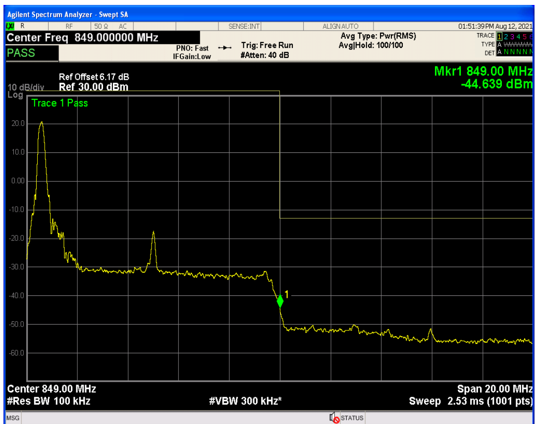
Band5 QAM16 BW=10MHz Channel=20600 RB Size=1 Position=#Max
