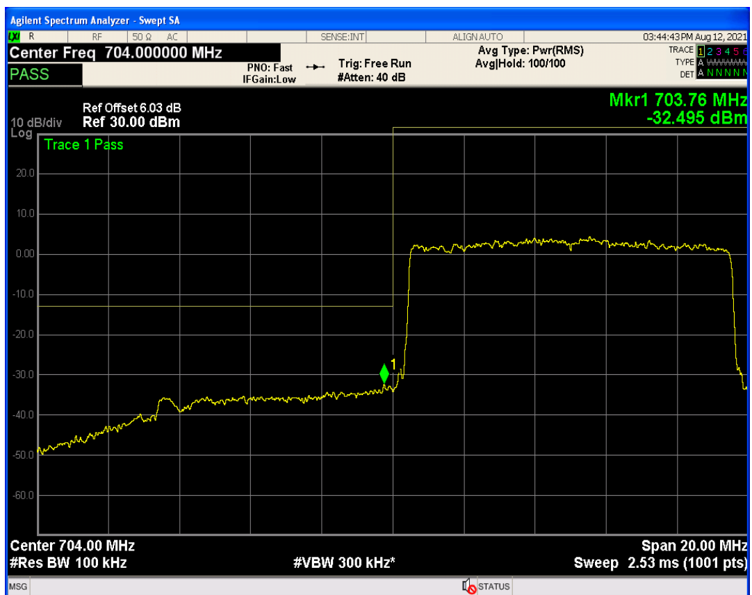
Band17 QPSK BW=10MHz Channel=23800 RB Size=1 Position=#0
