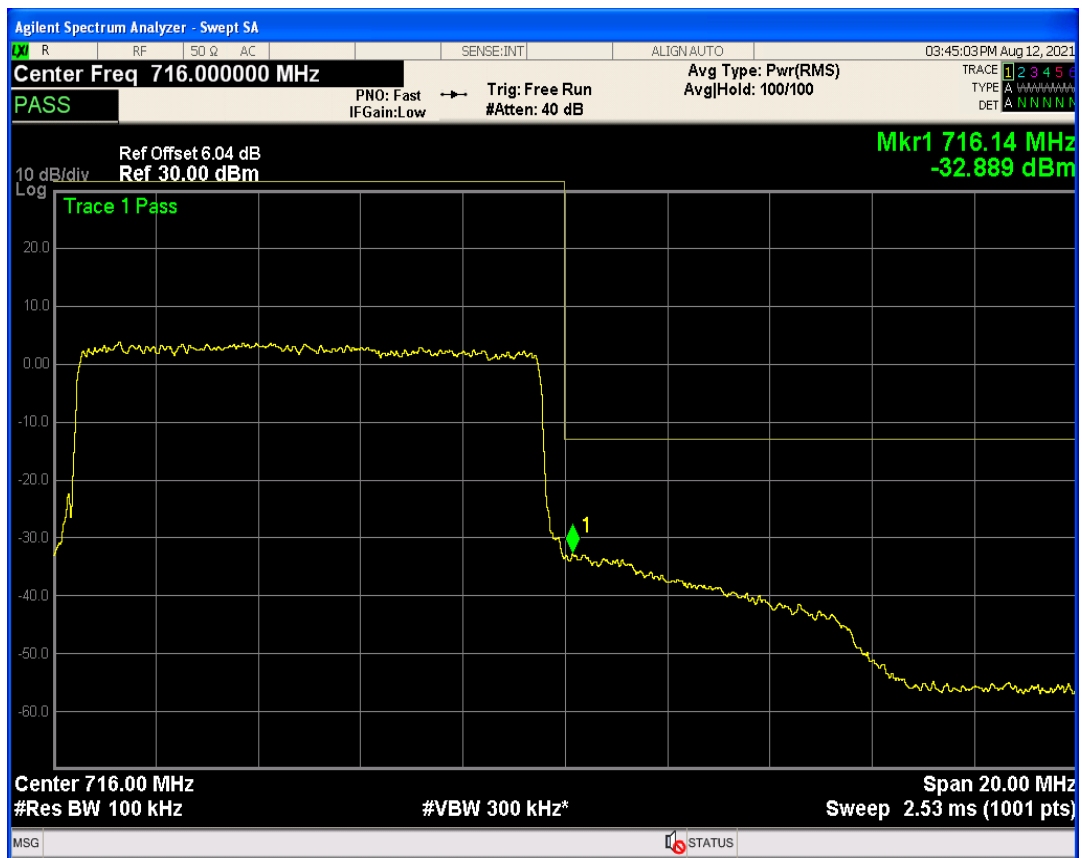
Band2 QPSK BW=1.4MHz Channel=18607 RB Size=1 Position=#0
