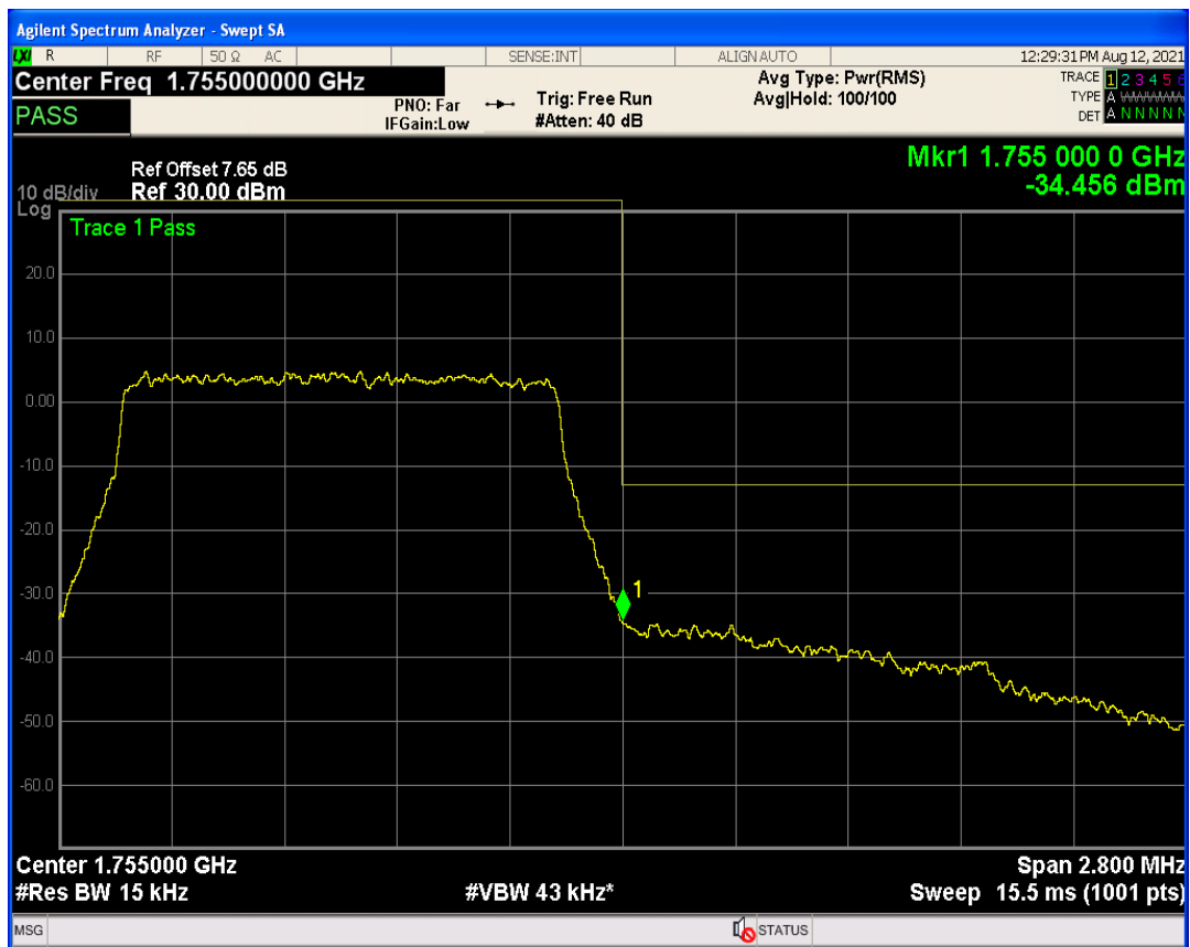
Band4 QPSK BW=3MHz Channel=19965 RB Size=1 Position=#Max
