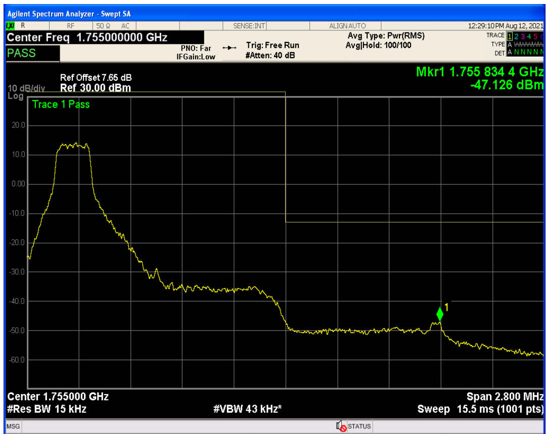
Band4 QPSK BW=1.4MHz Channel=20393 RB Size=1 Position=#Max
