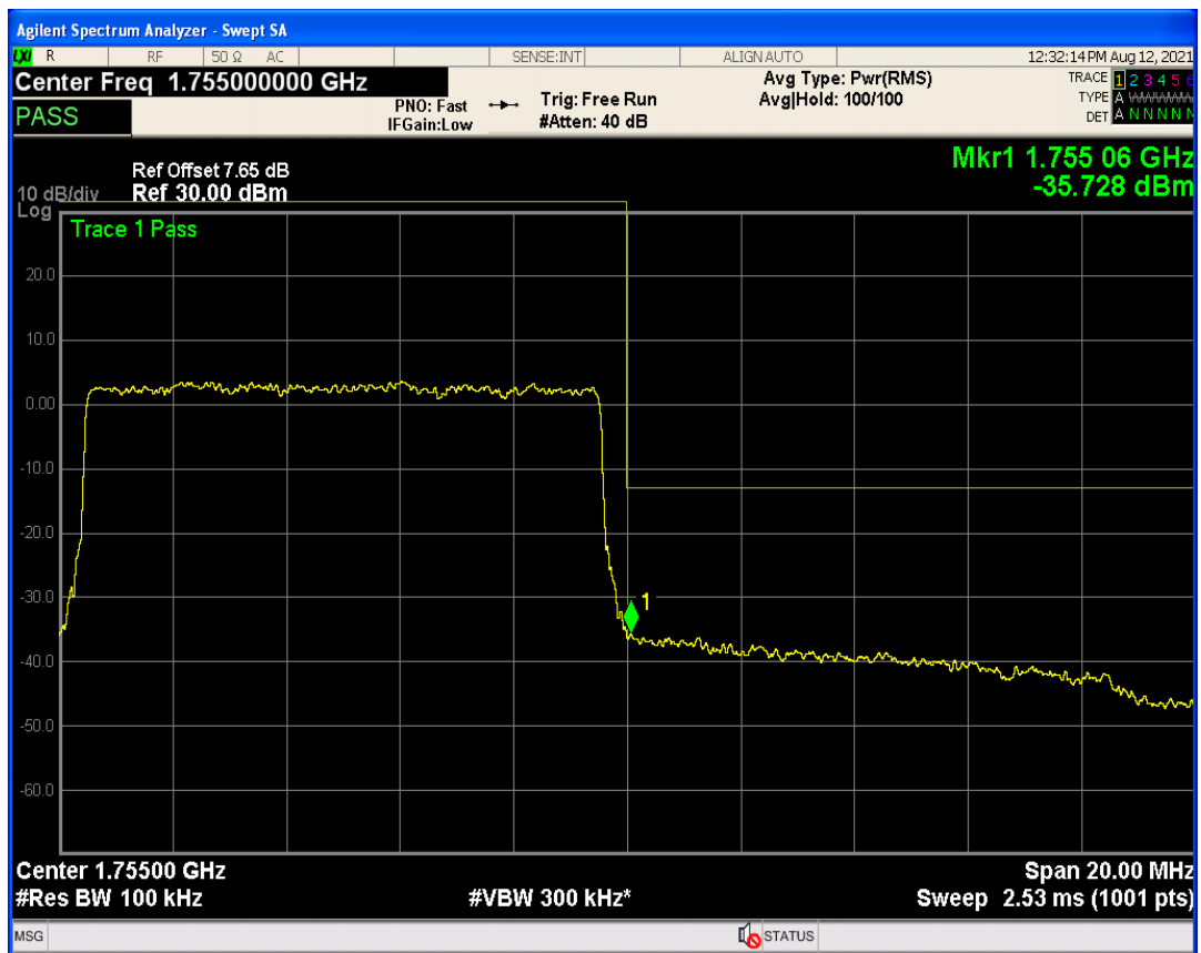
Band4 QPSK BW=15MHz Channel=20025 RB Size=1 Position=#Max
