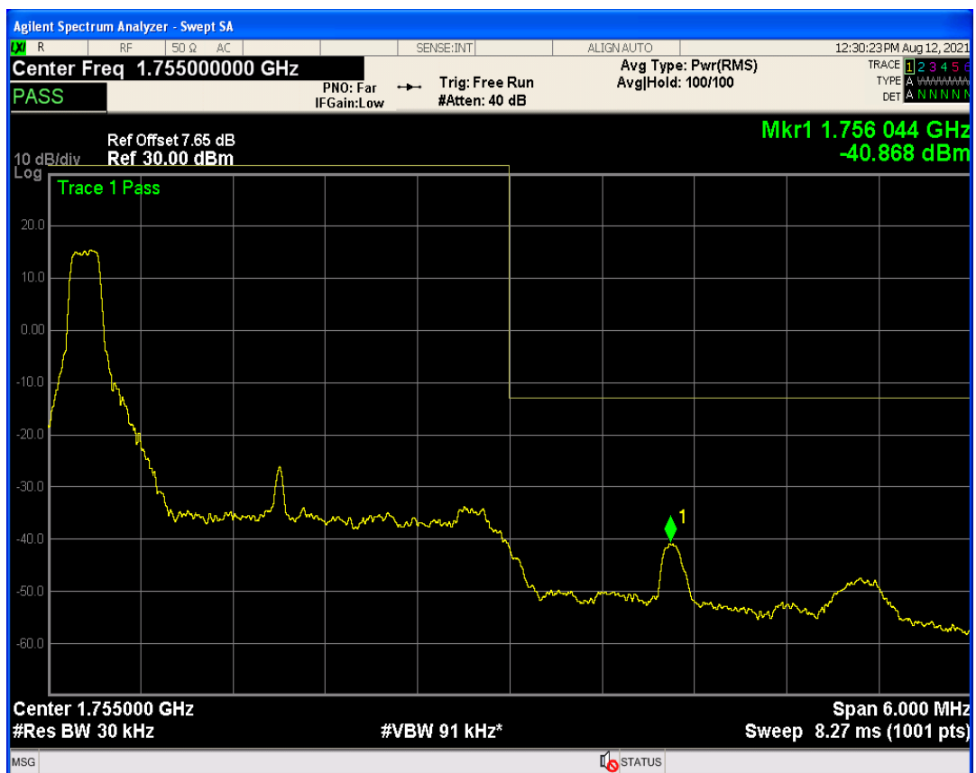
Band4 QAM16 BW=3MHz Channel=20385 RB Size=1 Position=#Max
