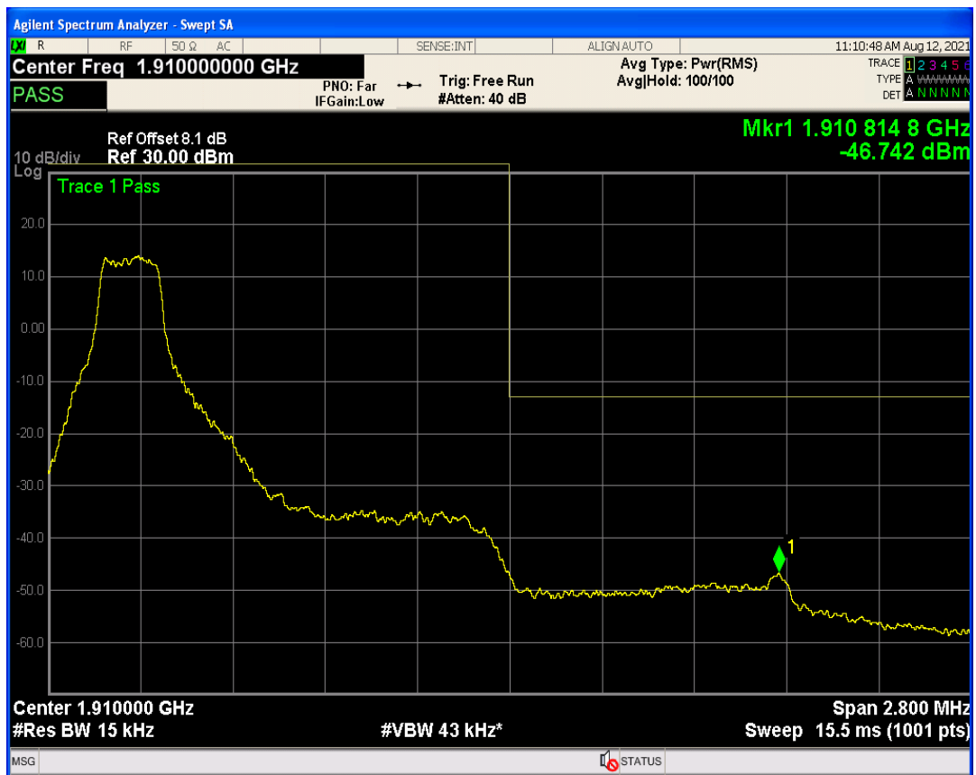
Band2 QPSK BW=1.4MHz Channel=19193 RB Size=1 Position=#Max
