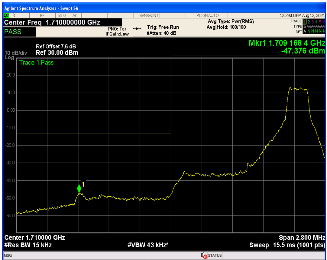
Band4 QAM16 BW=1.4MHz Channel=19957 RB Size=6 Position=#0
