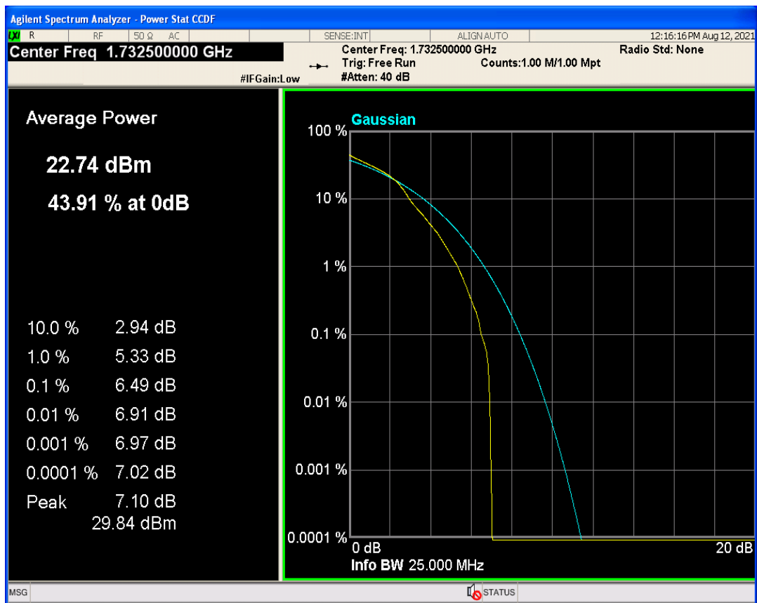
Band5 QPSK BW=1.4MHz Channel=20525 RB Size=1 Position=#0
