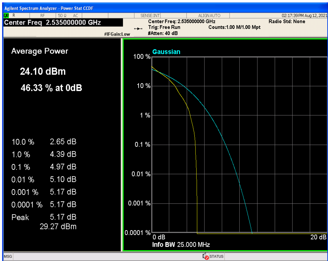
Band7 QAM16 BW=5MHz Channel=21100 RB Size=1 Position=#0
