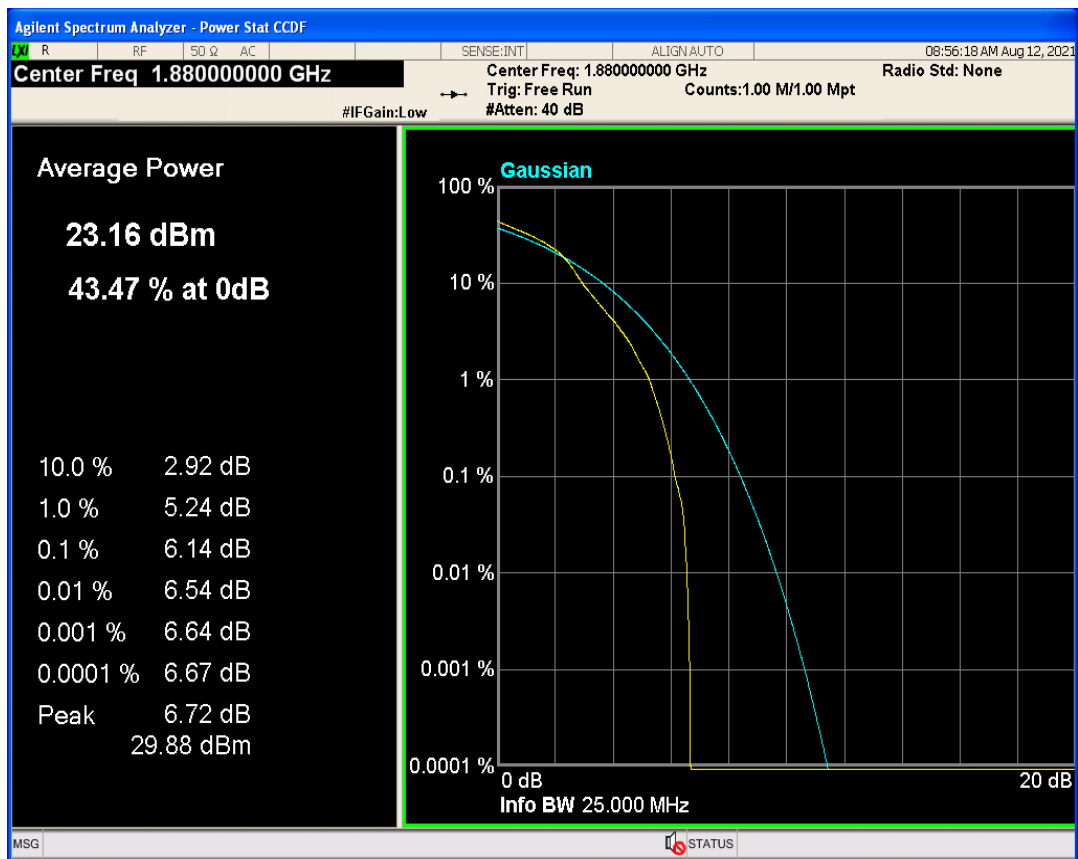
Band2 QPSK BW=20MHz Channel=18900 RB Size=1 Position=#0
