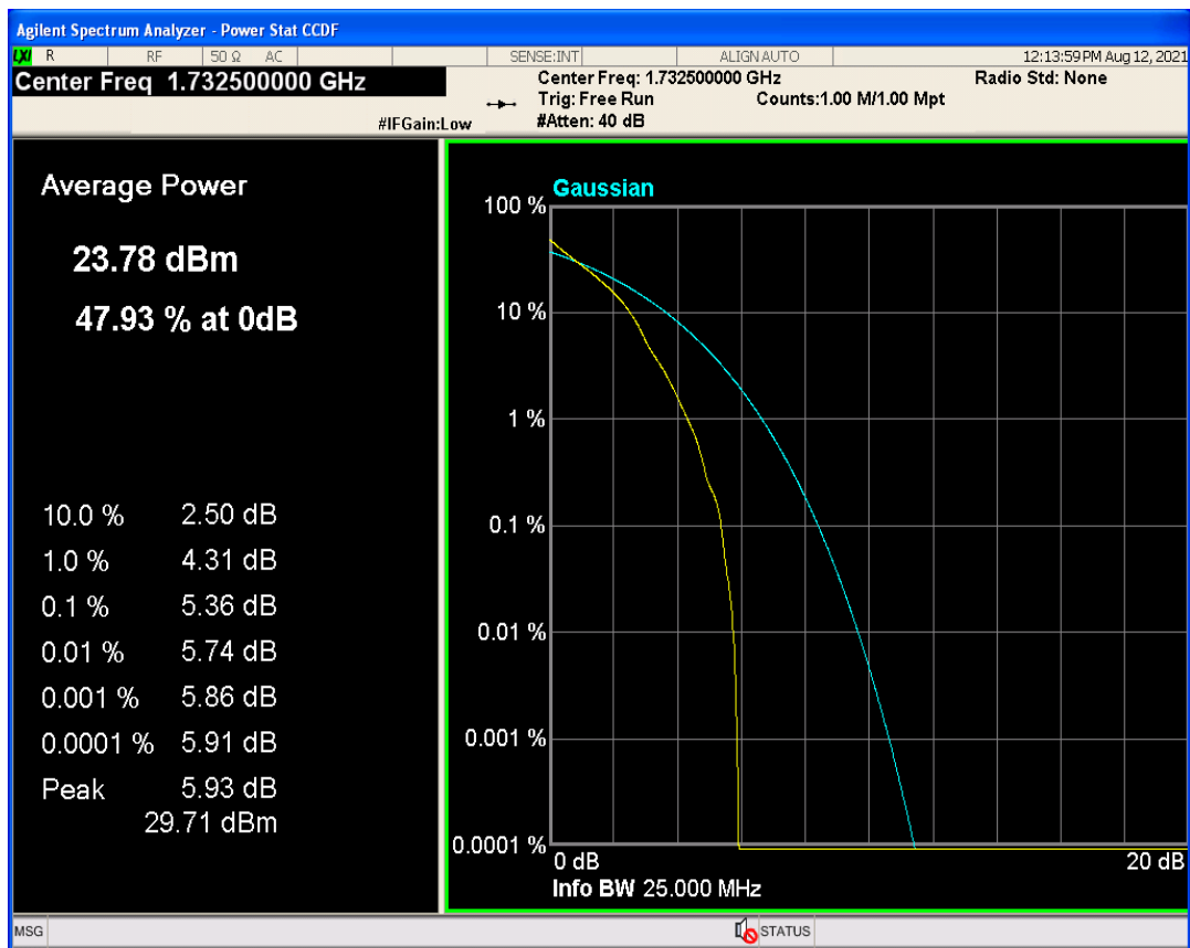
Band4 QAM16 BW=15MHz Channel=20175 RB Size=1 Position=#0
