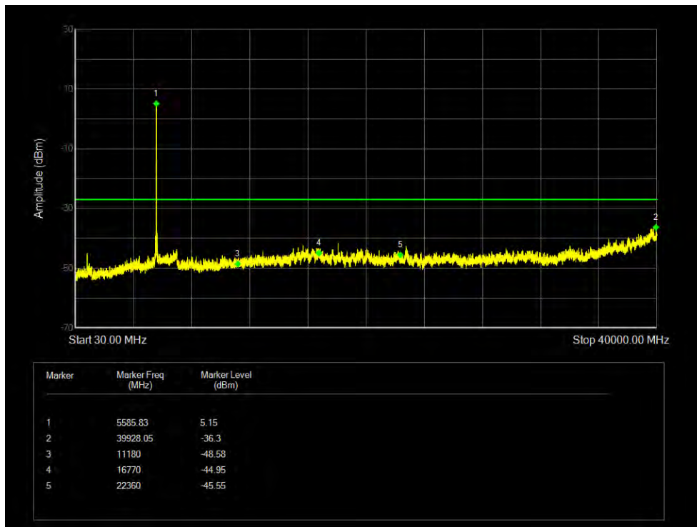
Tx. Spurious NVNT 802.11n(HT40) 5670MHz Ant1 Emission
