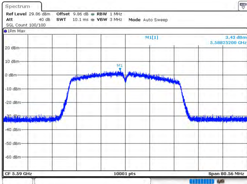
PSD NVNT 802.11ac40 5590MHz Ant1
