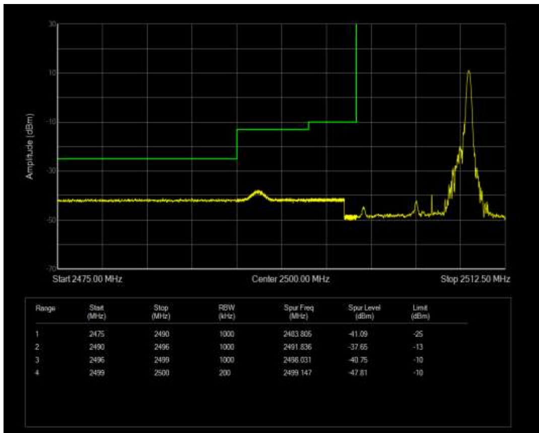
Band7 QPSK BW=10MHz Channel=20800 RB Size=50 Position=#0
