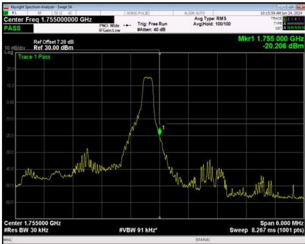
Band4 16QAM BW=3MHz Channel=20385 RB Size=15 Position=#0
