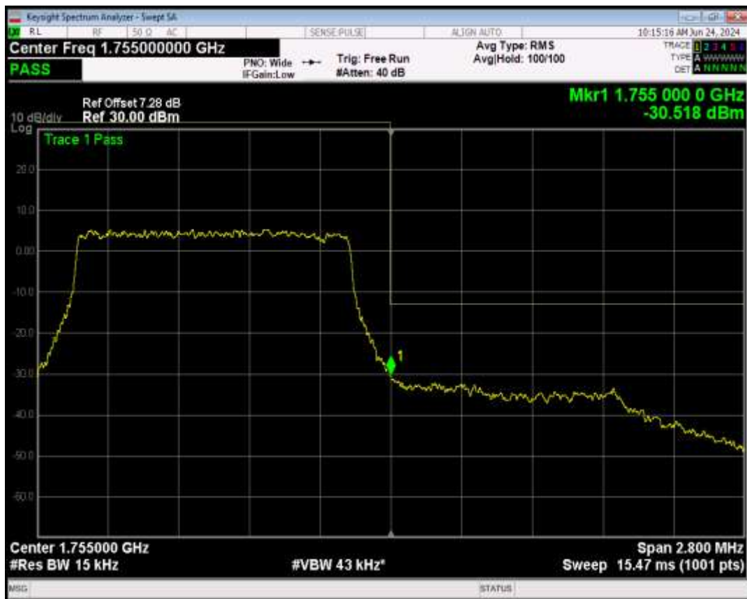
Band4 16QAM BW=1.4MHz Channel=20393 RB Size=1 Position=#0
