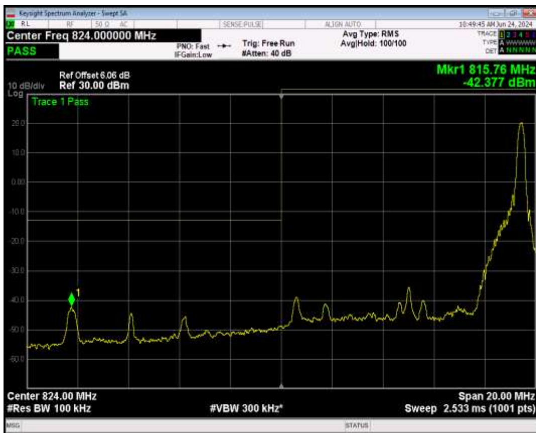
Band5 QPSK BW=10MHz Channel=20450 RB Size=50 Position=#0
