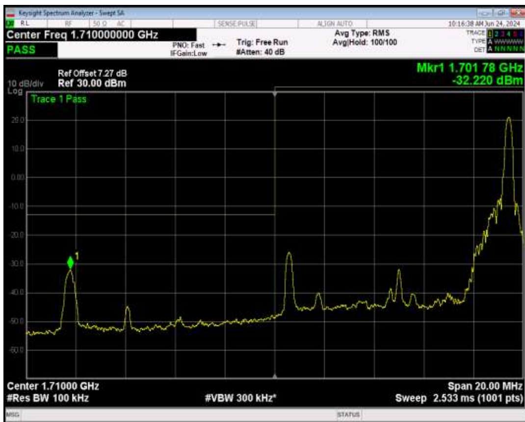
Band4 QPSK BW=10MHz Channel=20000 RB Size=50 Position=#0
