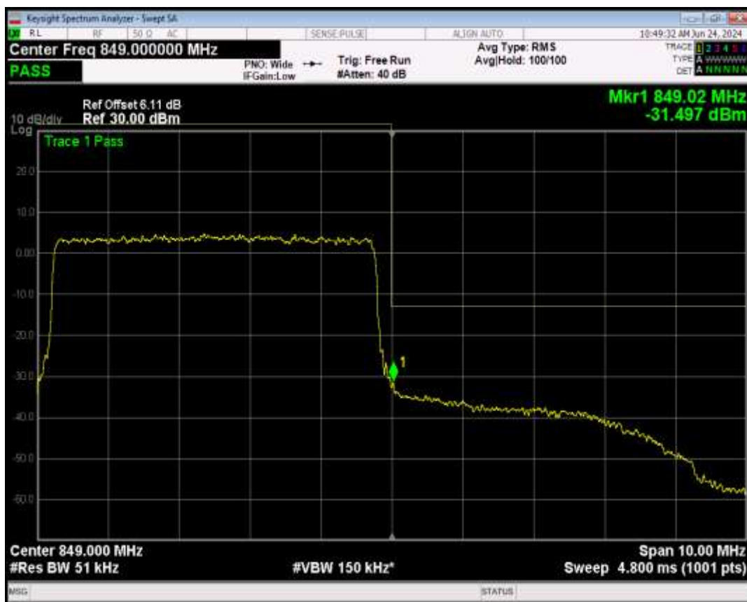
Band5 16QAM BW=5MHz Channel=20625 RB Size=1 Position=#0
