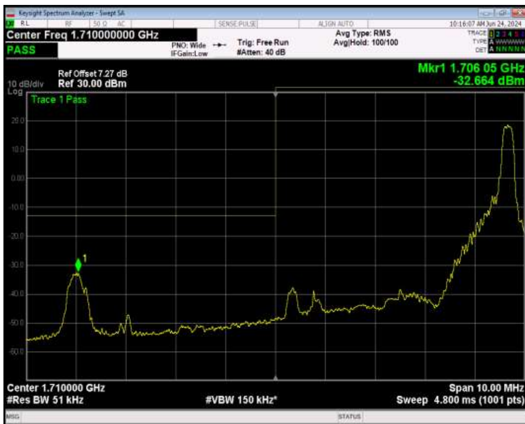
Band4 QPSK BW=5MHz Channel=19975 RB Size=25 Position=#0
