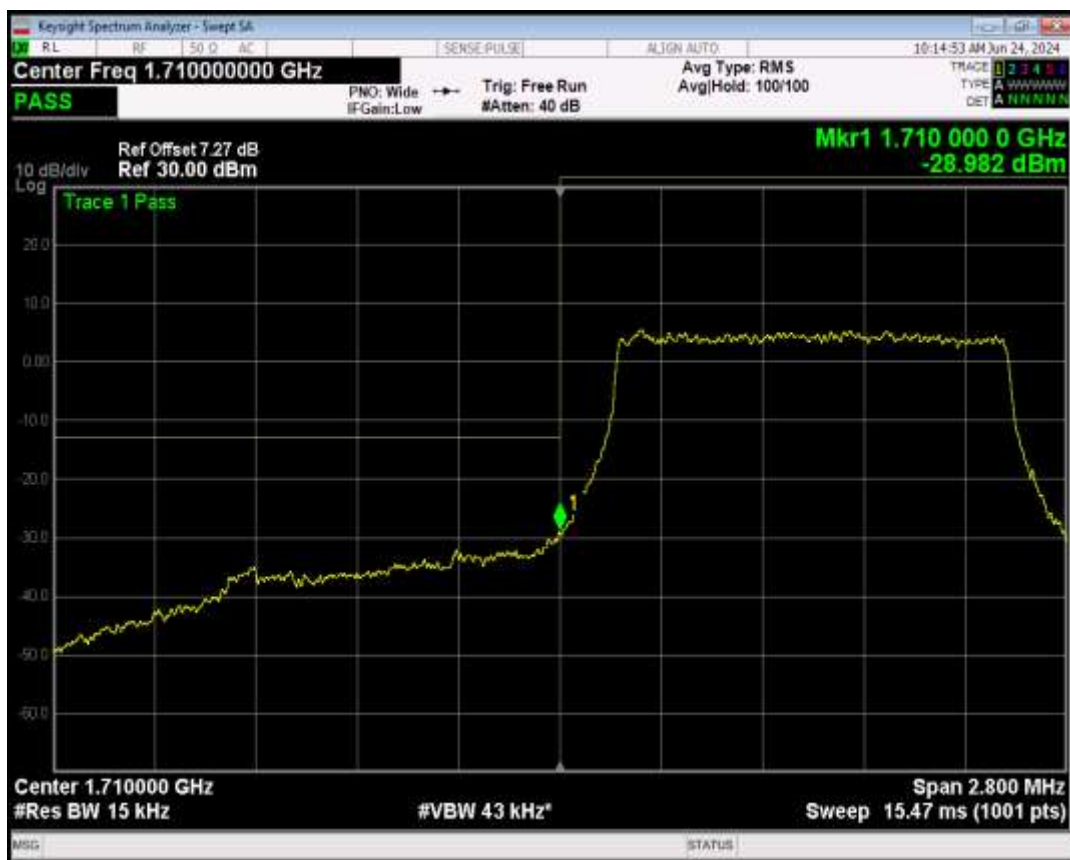
Band4 16QAM BW=1.4MHz Channel=19957 RB Size=1 Position=#0
