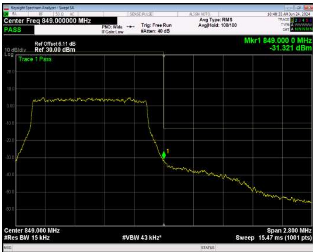
Band5 QPSK BW=3MHz Channel=20415 RB Size=1 Position=#0
