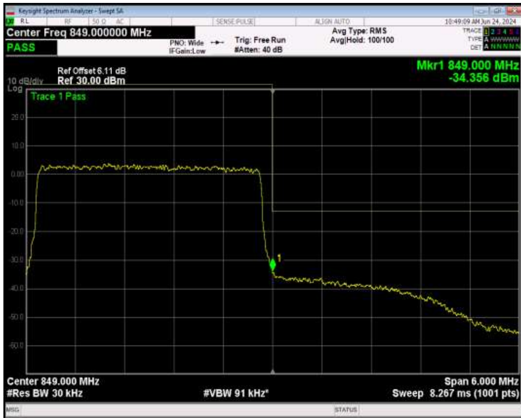
Band5 QPSK BW=5MHz Channel=20425 RB Size=1 Position=#0
