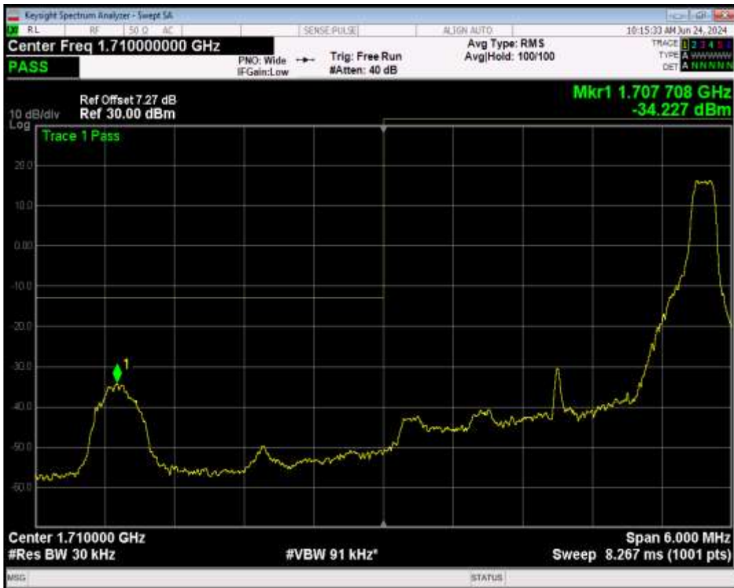
Band4 16QAM BW=3MHz Channel=19965 RB Size=1 Position=#0
