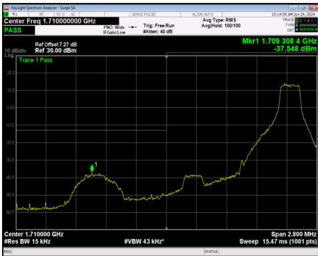
Band4 QPSK BW=1.4MHz Channel=19957 RB Size=6 Position=#0
