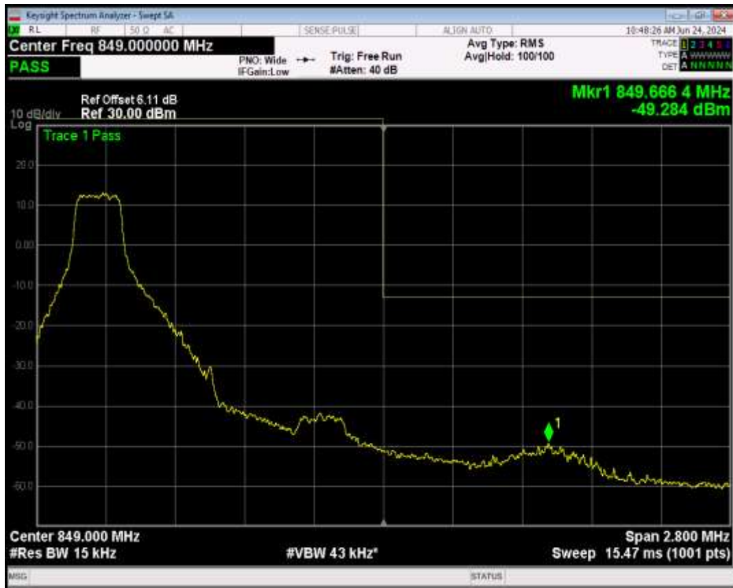
Band5 16QAM BW=1.4MHz Channel=20643 RB Size=1 Position=#Max
