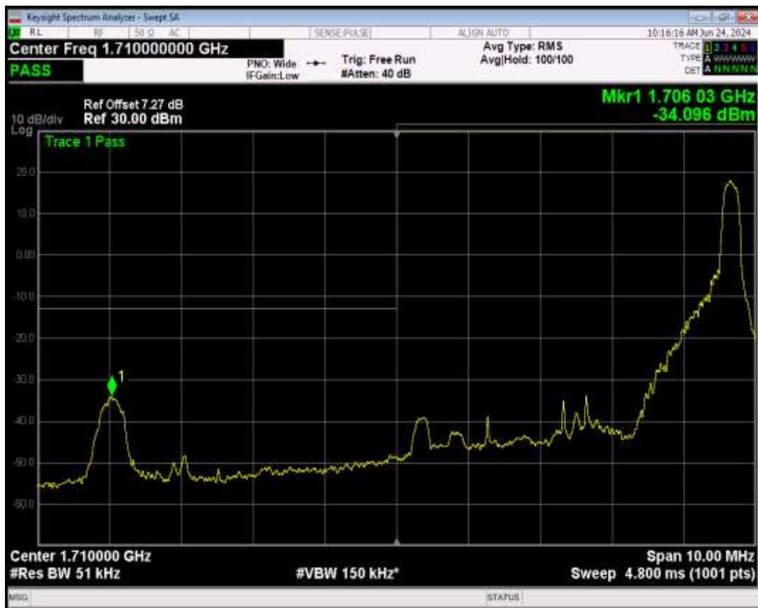
Band4 16QAM BW=5MHz Channel=19975 RB Size=25 Position=#0
