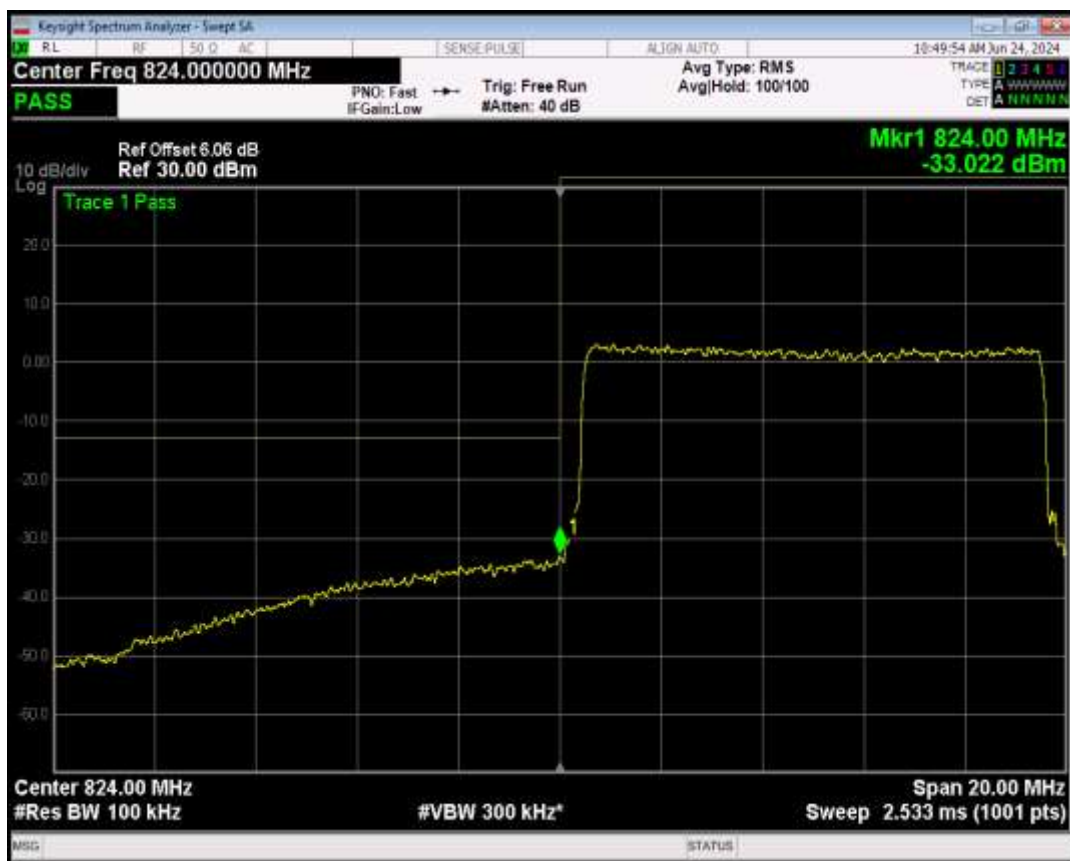
Band5 QPSK BW=10MHz Channel=20600 RB Size=1 Position=#0
