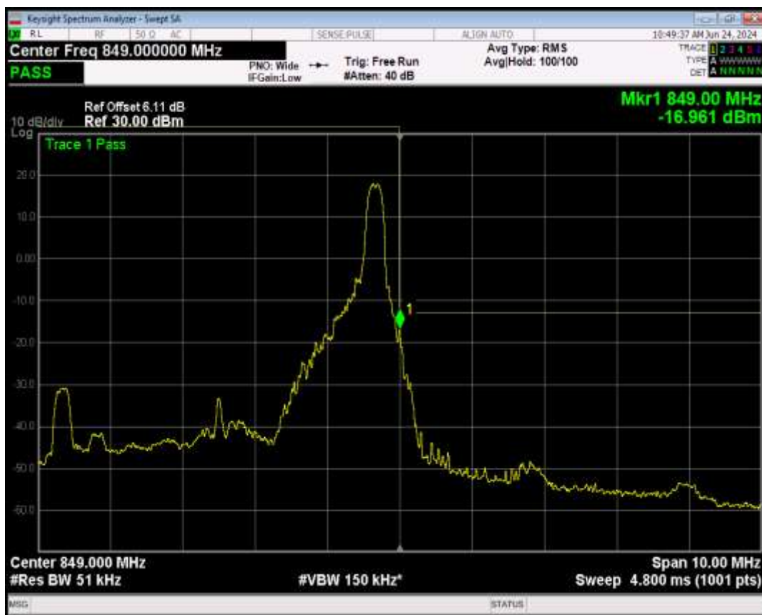
Band5 QPSK BW=10MHz Channel=20450 RB Size=1 Position=#0
