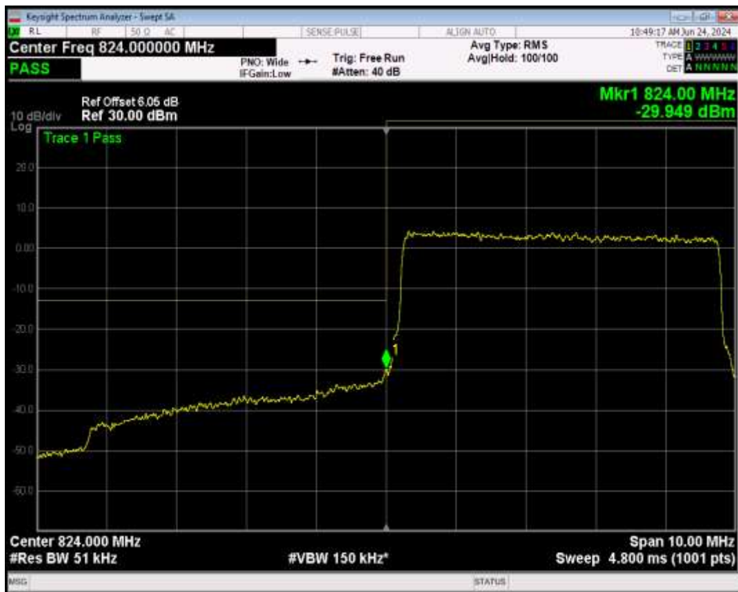
Band5 16QAM BW=5MHz Channel=20425 RB Size=1 Position=#0
