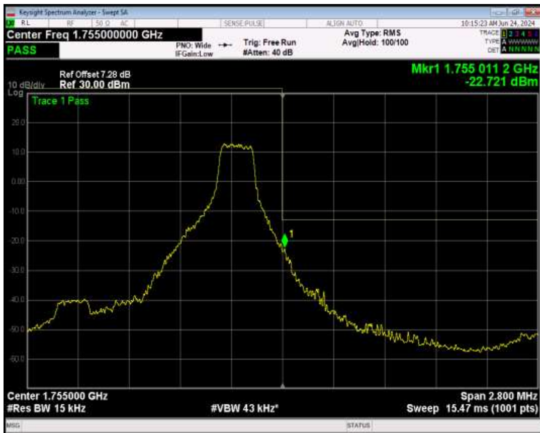
Band4 16QAM BW=1.4MHz Channel=20393 RB Size=6 Position=#0
