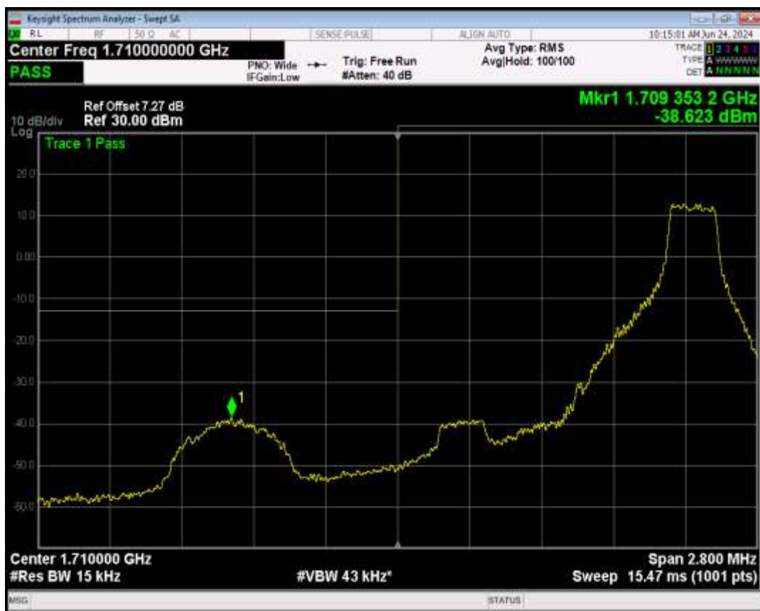
Band4 16QAM BW=1.4MHz Channel=19957 RB Size=6 Position=#0
