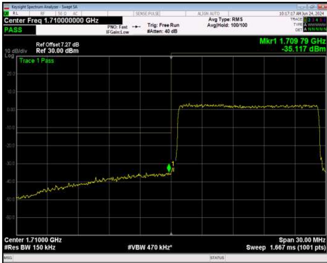
Band4 QPSK BW=15MHz Channel=20325 RB Size=1 Position=#0
