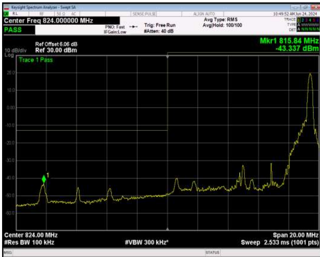
Band5 16QAM BW=10MHz Channel=20450 RB Size=50 Position=#0
