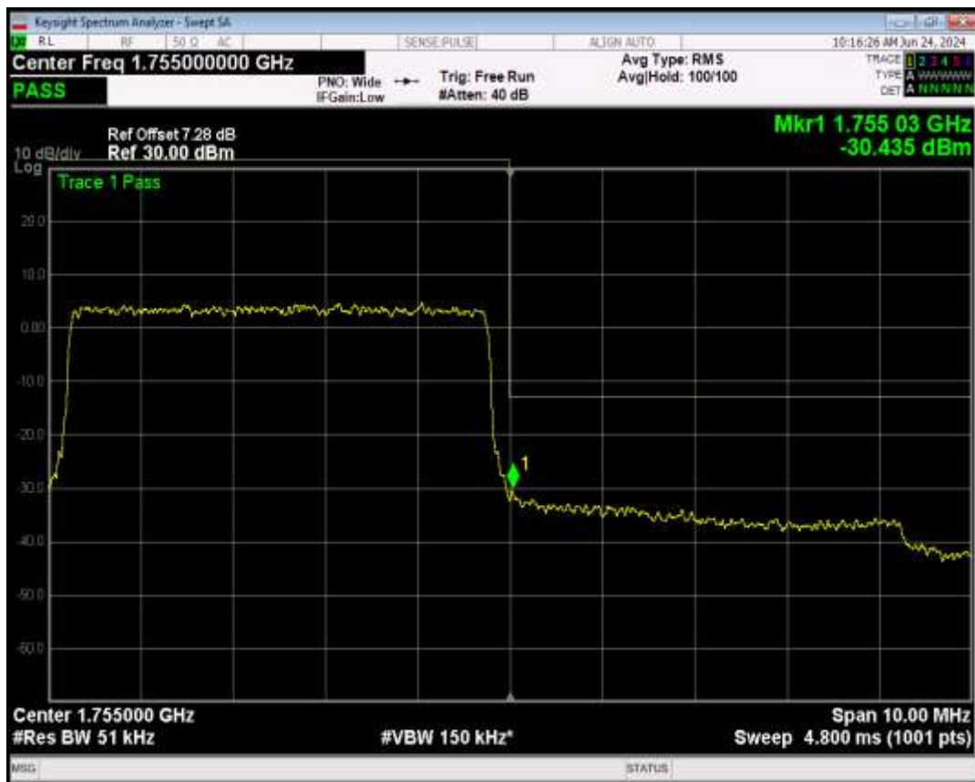
Band4 16QAM BW=5MHz Channel=20375 RB Size=1 Position=#0
