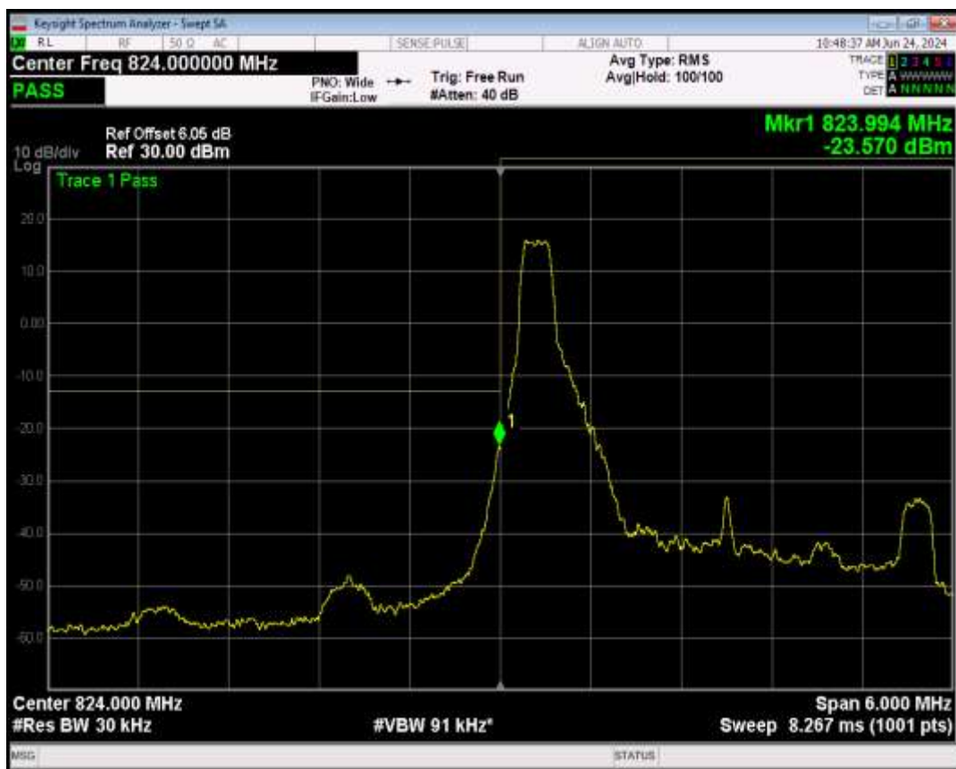
Band5 QPSK BW=3MHz Channel=20415 RB Size=1 Position=#Max
