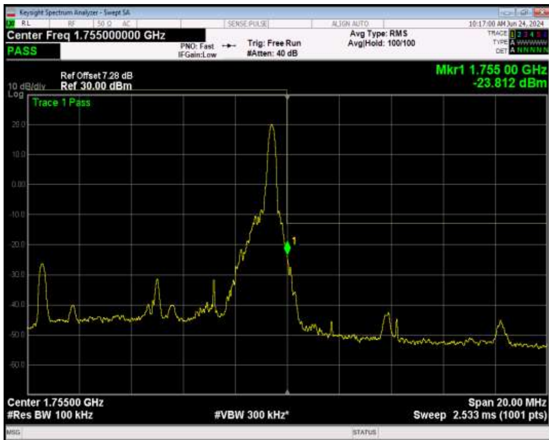
Band4 16QAM BW=10MHz Channel=20350 RB Size=50 Position=#0
