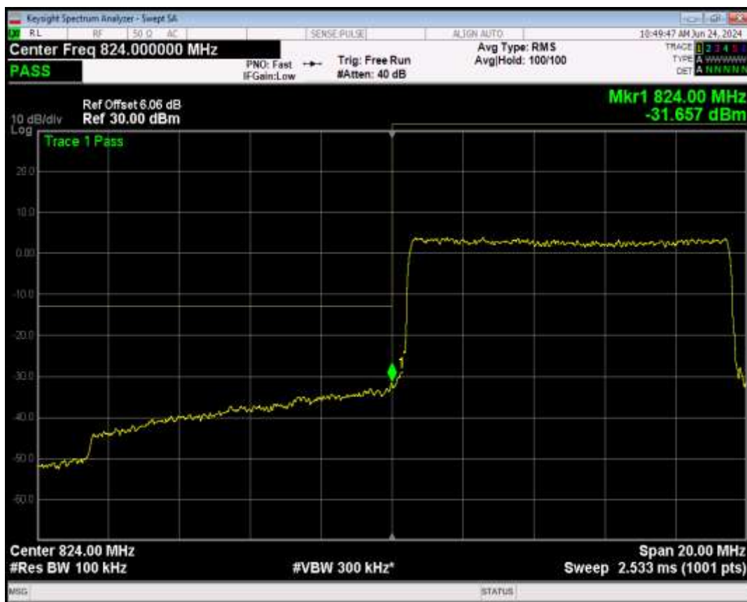
Band5 16QAM BW=10MHz Channel=20450 RB Size=1 Position=#0
