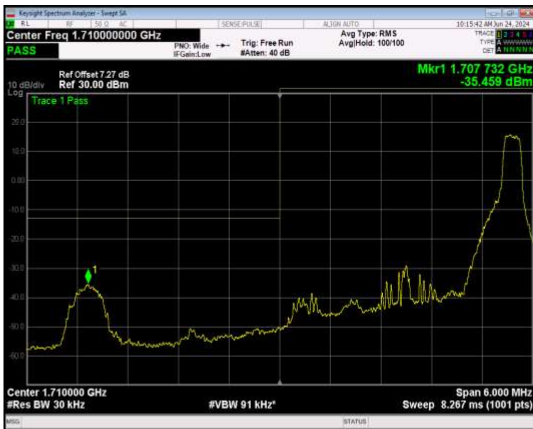
Band4 16QAM BW=3MHz Channel=19965 RB Size=15 Position=#0
