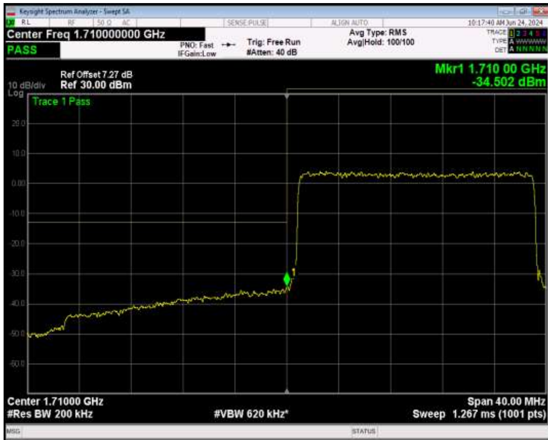
Band4 16QAM BW=20MHz Channel=20050 RB Size=1 Position=#Max
