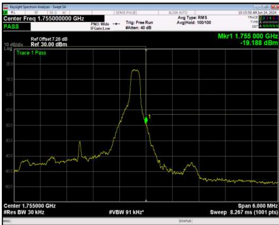
Band4 QPSK BW=3MHz Channel=20385 RB Size=15 Position=#0
