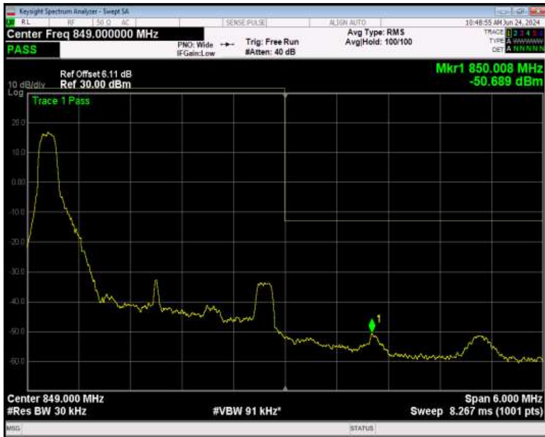
Band5 QPSK BW=3MHz Channel=20635 RB Size=15 Position=#0
