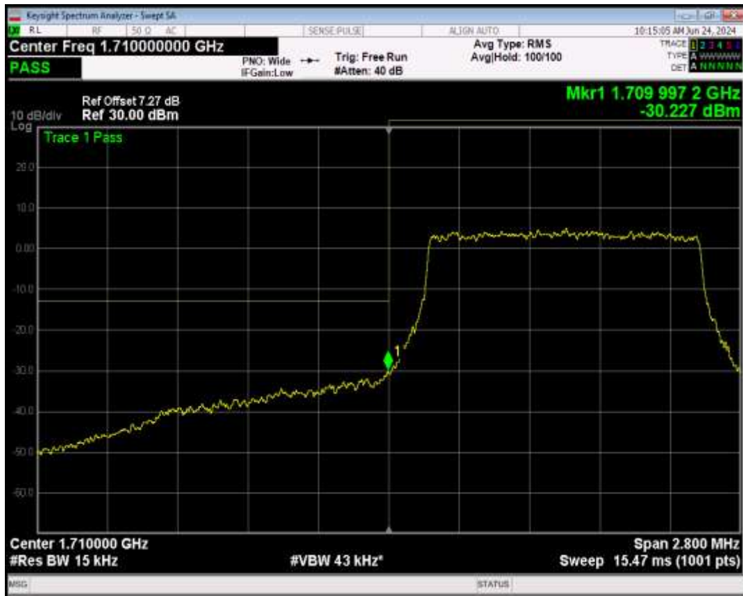
Band4 QPSK BW=1.4MHz Channel=20393 RB Size=1 Position=#0
