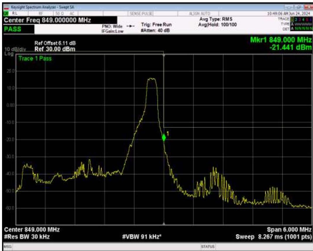
Band5 16QAM BW=3MHz Channel=20635 RB Size=15 Position=#0
