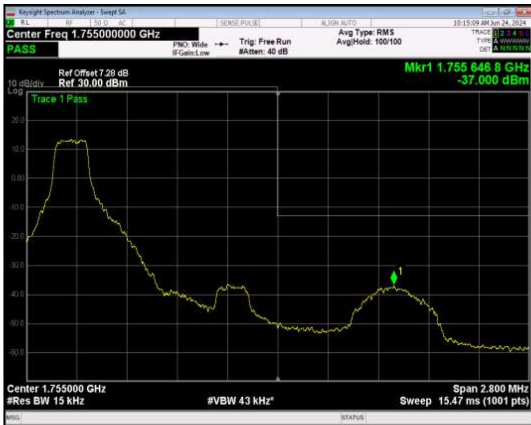
Band4 QPSK BW=1.4MHz Channel=20393 RB Size=1 Position=#Max
