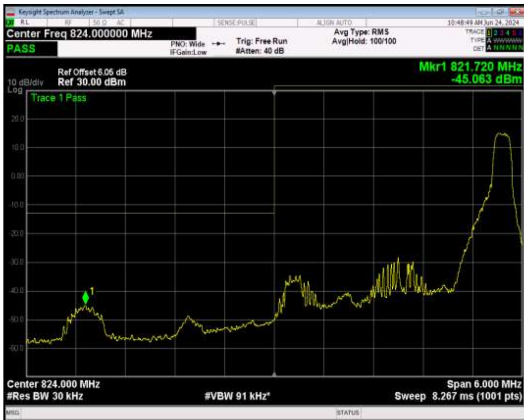
Band5 16QAM BW=3MHz Channel=20415 RB Size=15 Position=#0
