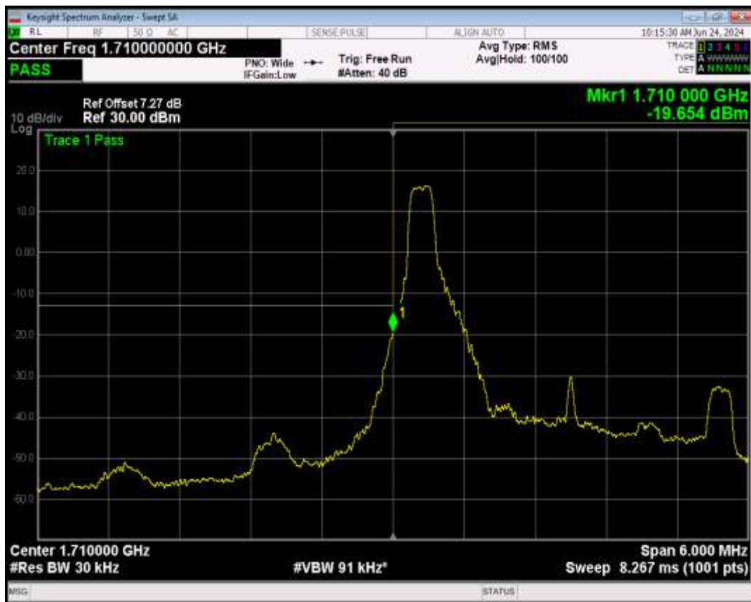
Band4 QPSK BW=3MHz Channel=19965 RB Size=15 Position=#0
