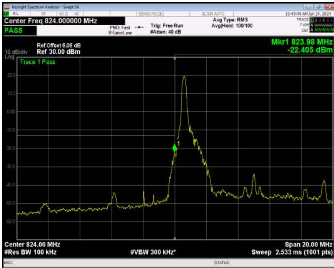
Band5 16QAM BW=10MHz Channel=20450 RB Size=1 Position=#Max
