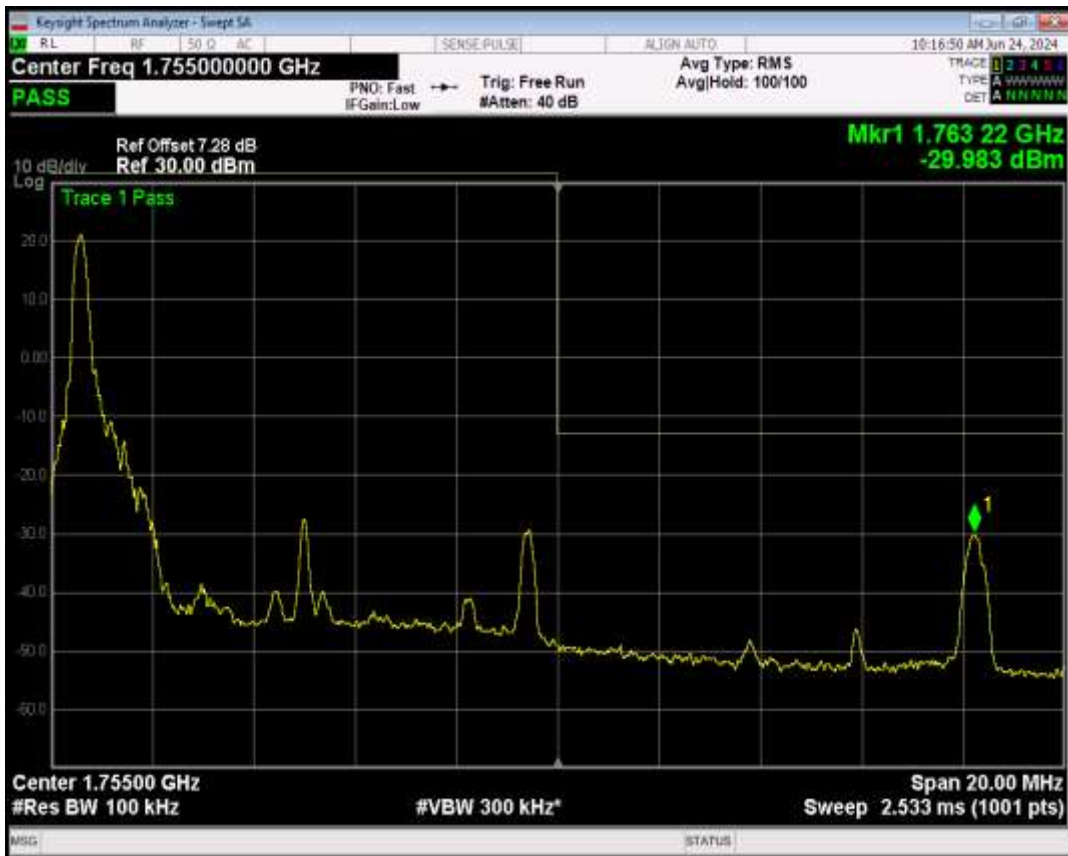
Band4 QPSK BW=10MHz Channel=20350 RB Size=1 Position=#Max
