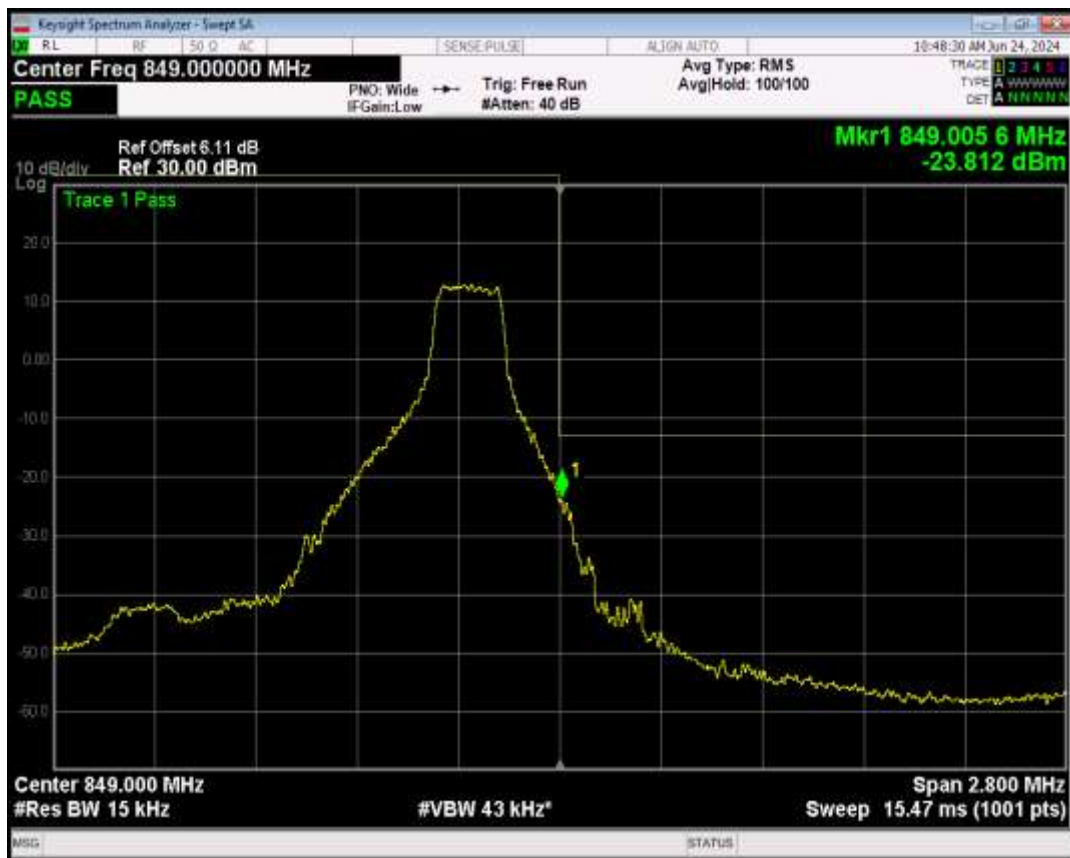
Band5 16QAM BW=1.4MHz Channel=20643 RB Size=6 Position=#0
