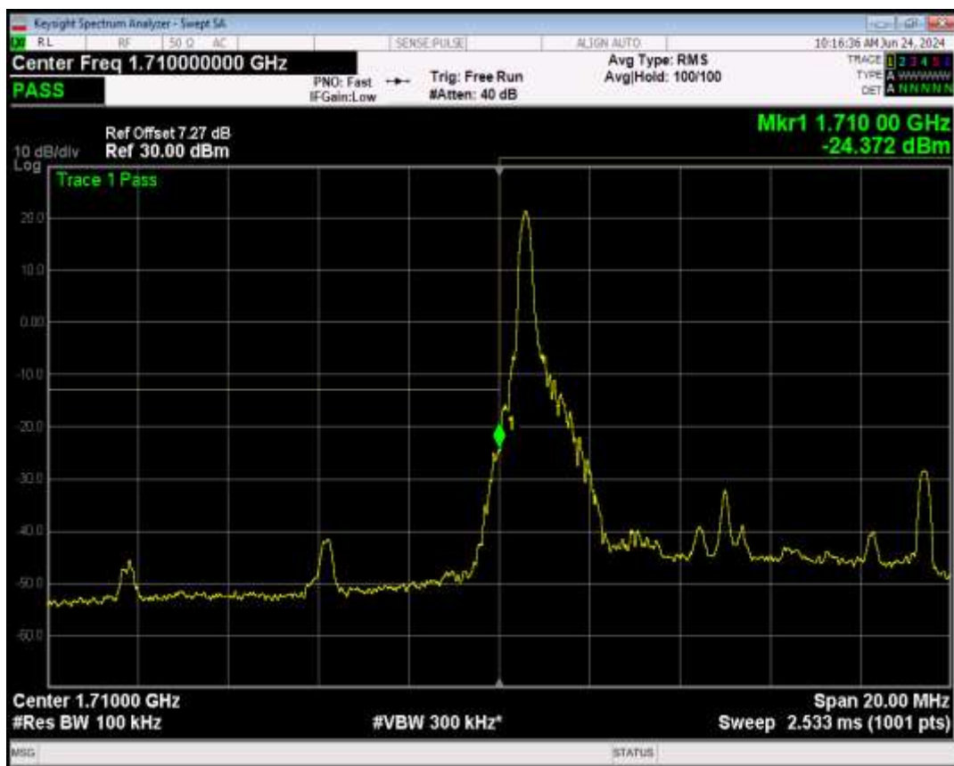
Band4 QPSK BW=10MHz Channel=20000 RB Size=1 Position=#Max
