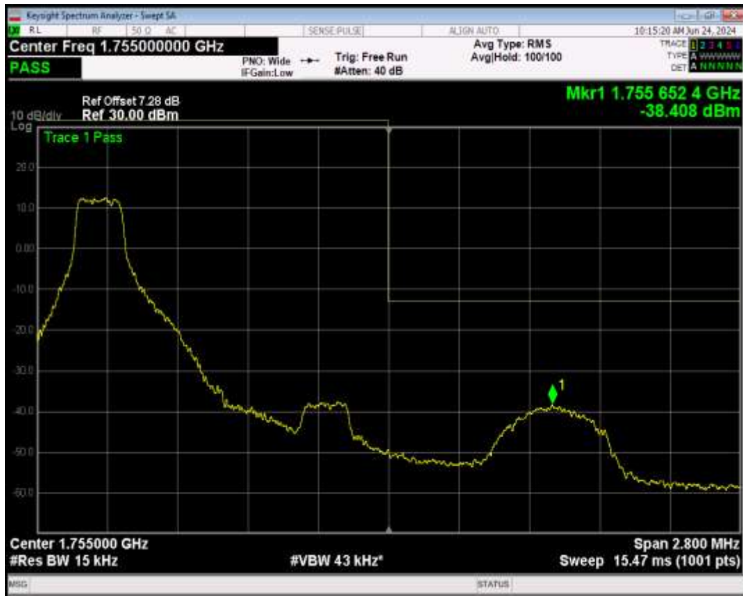
Band4 16QAM BW=1.4MHz Channel=20393 RB Size=1 Position=#Max
