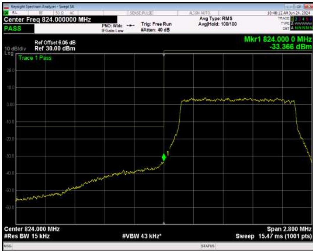
Band5 QPSK BW=1.4MHz Channel=20643 RB Size=1 Position=#0
