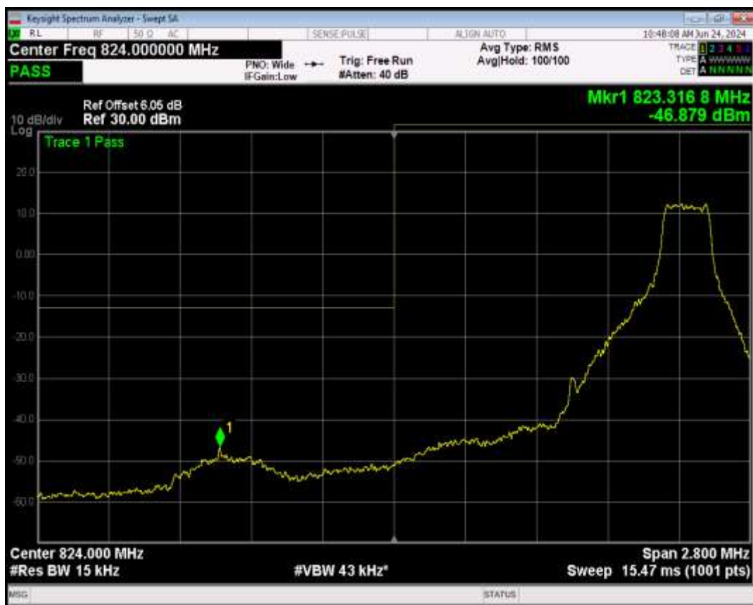
Band5 16QAM BW=1.4MHz Channel=20407 RB Size=6 Position=#0
