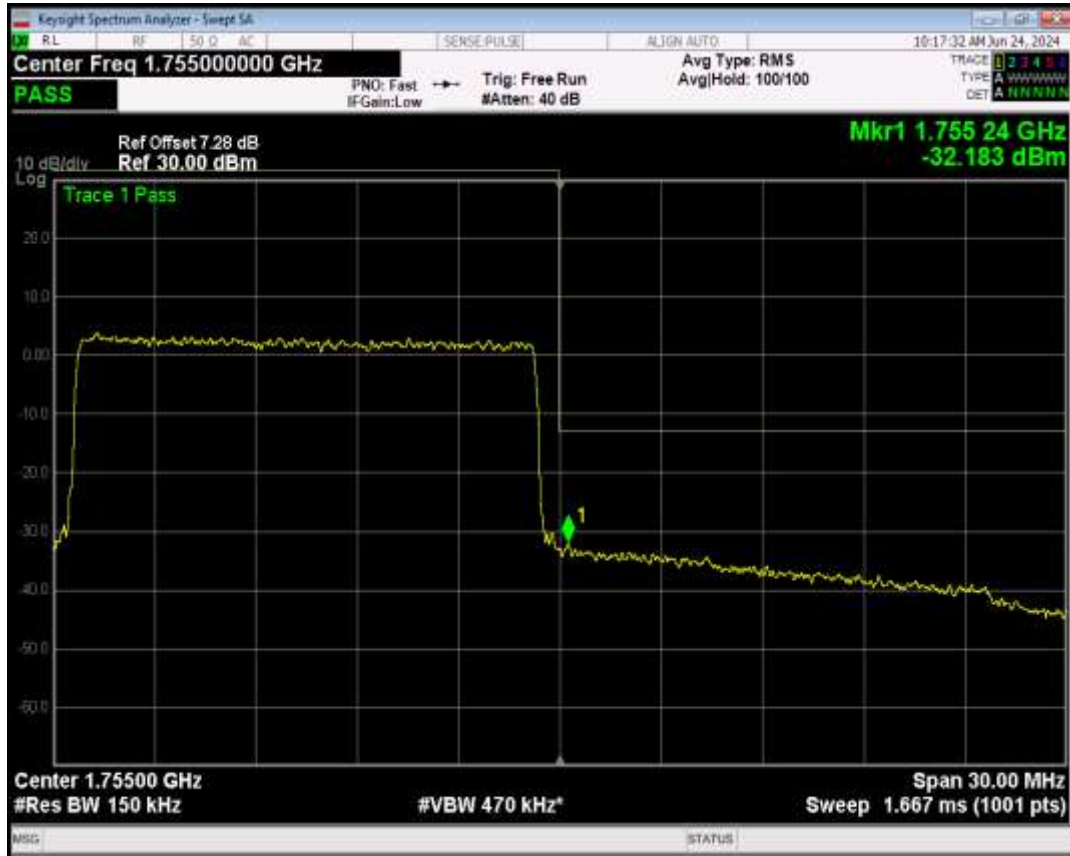
Band4 QPSK BW=20MHz Channel=20050 RB Size=1 Position=#0
