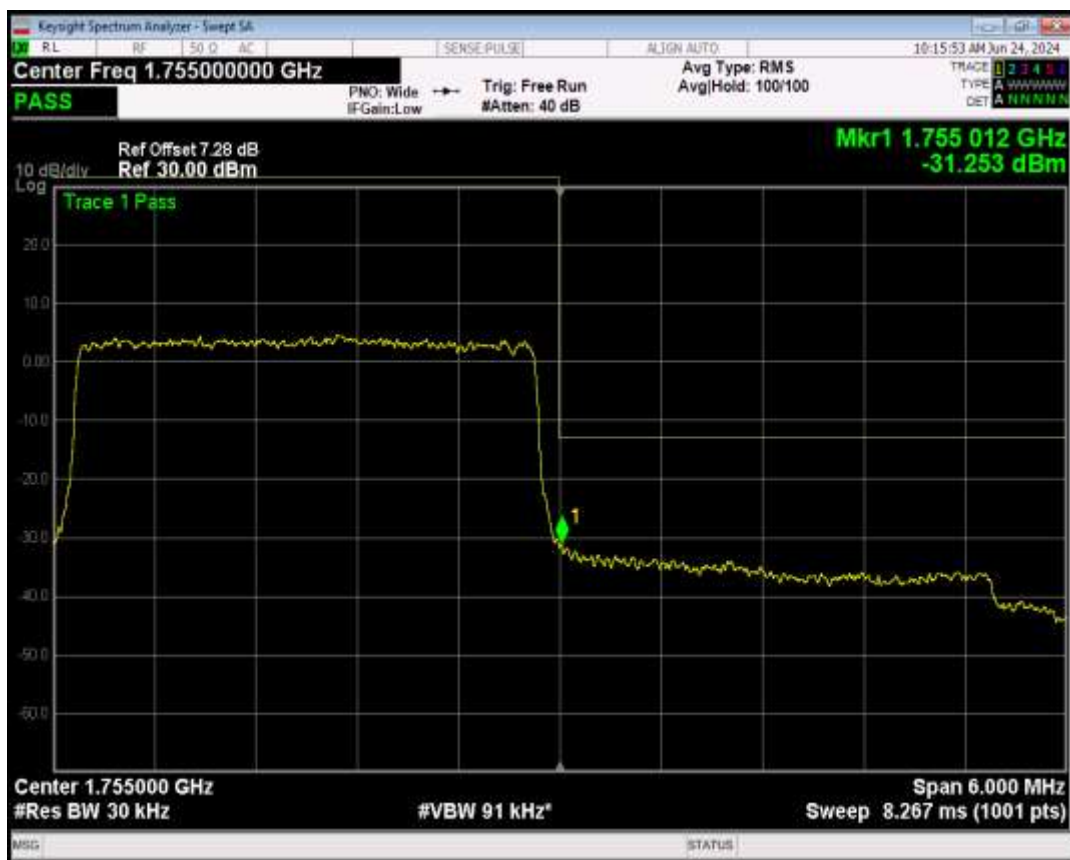
Band4 16QAM BW=3MHz Channel=20385 RB Size=1 Position=#0
