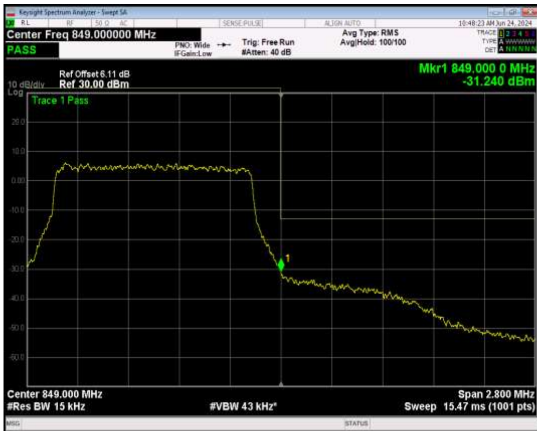
Band5 16QAM BW=1.4MHz Channel=20643 RB Size=1 Position=#0
