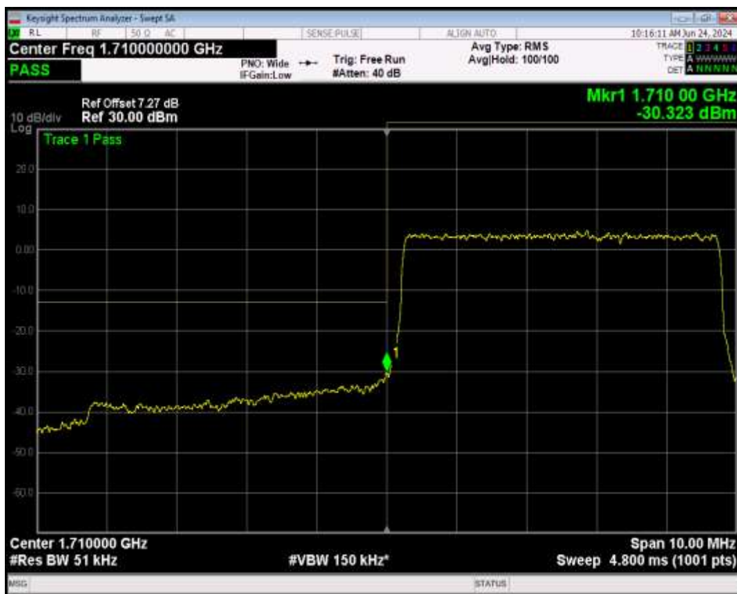
Band4 16QAM BW=5MHz Channel=19975 RB Size=1 Position=#0
