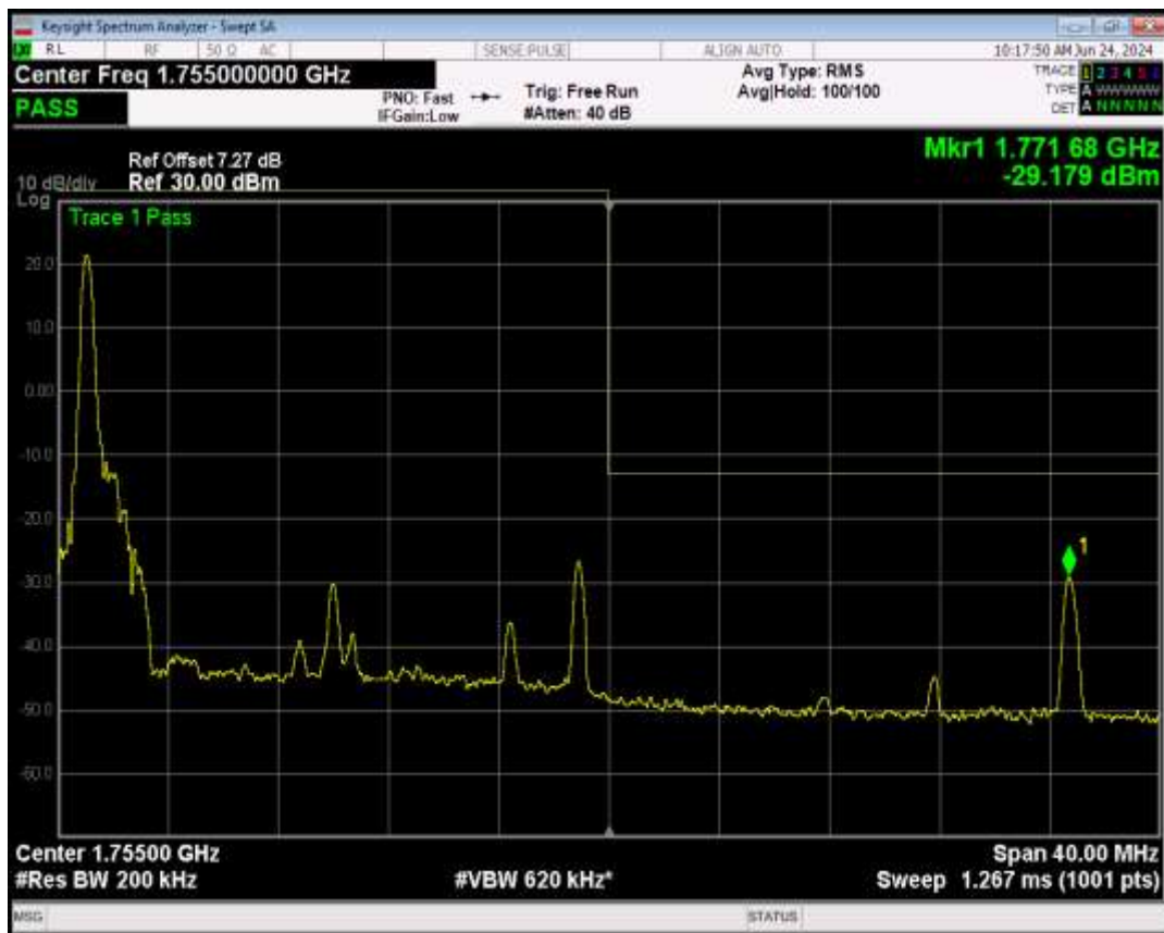
Band4 QPSK BW=20MHz Channel=20300 RB Size=1 Position=#Max
