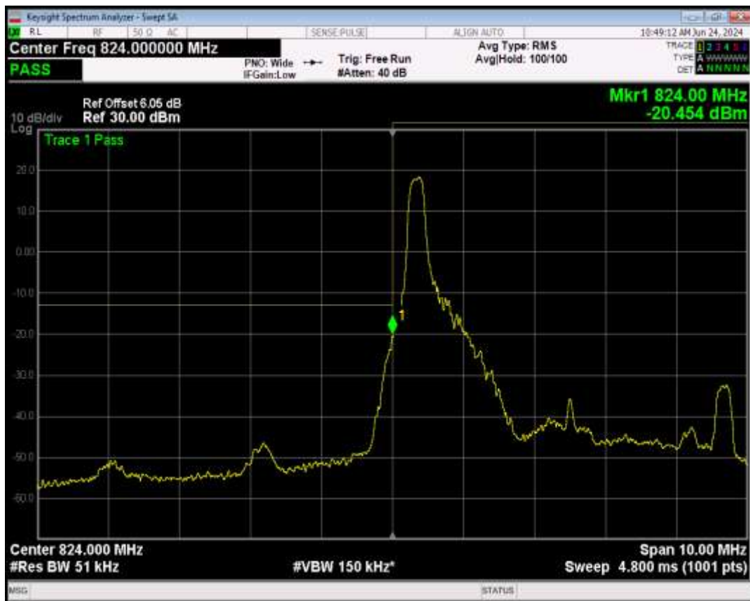
Band5 QPSK BW=5MHz Channel=20425 RB Size=1 Position=#Max
