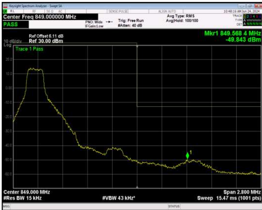
Band5 QPSK BW=1.4MHz Channel=20643 RB Size=1 Position=#Max
