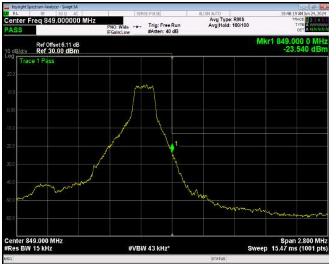
Band5 QPSK BW=1.4MHz Channel=20643 RB Size=6 Position=#0
