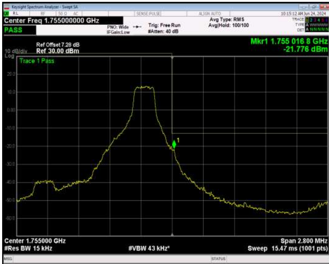
Band4 QPSK BW=1.4MHz Channel=20393 RB Size=6 Position=#0
