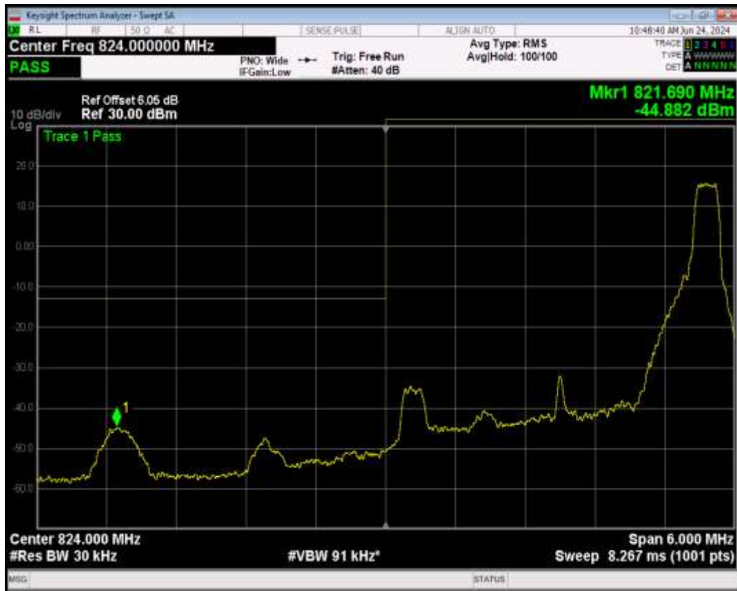
Band5 QPSK BW=3MHz Channel=20415 RB Size=15 Position=#0
