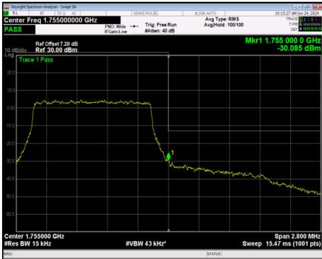
Band4 QPSK BW=3MHz Channel=19965 RB Size=1 Position=#0
