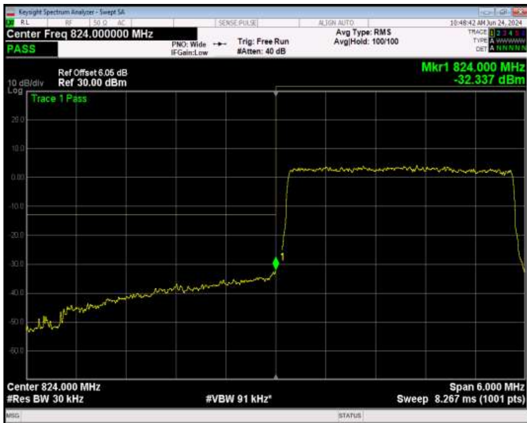
Band5 16QAM BW=3MHz Channel=20415 RB Size=1 Position=#0
