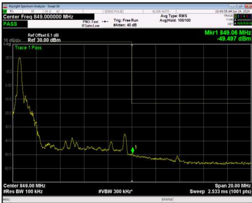
Band5 QPSK BW=10MHz Channel=20600 RB Size=1 Position=#Max
