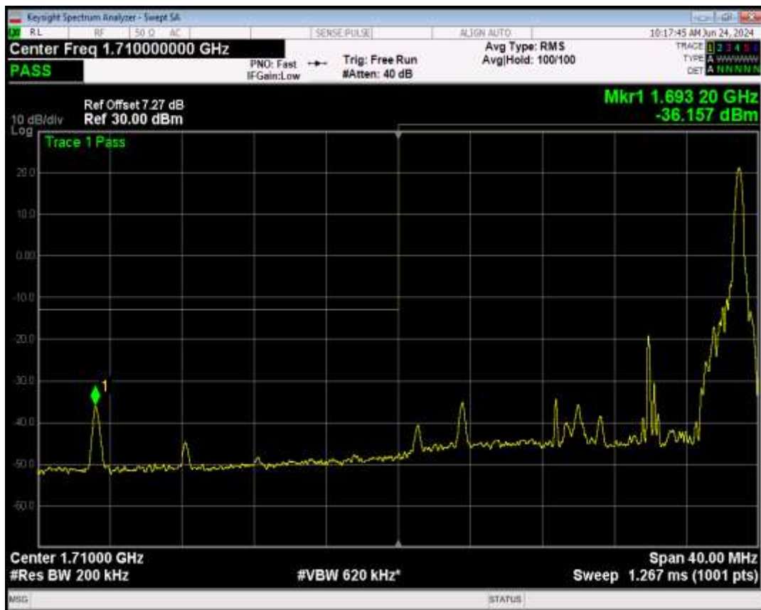
Band4 16QAM BW=20MHz Channel=20050 RB Size=100 Position=#0
