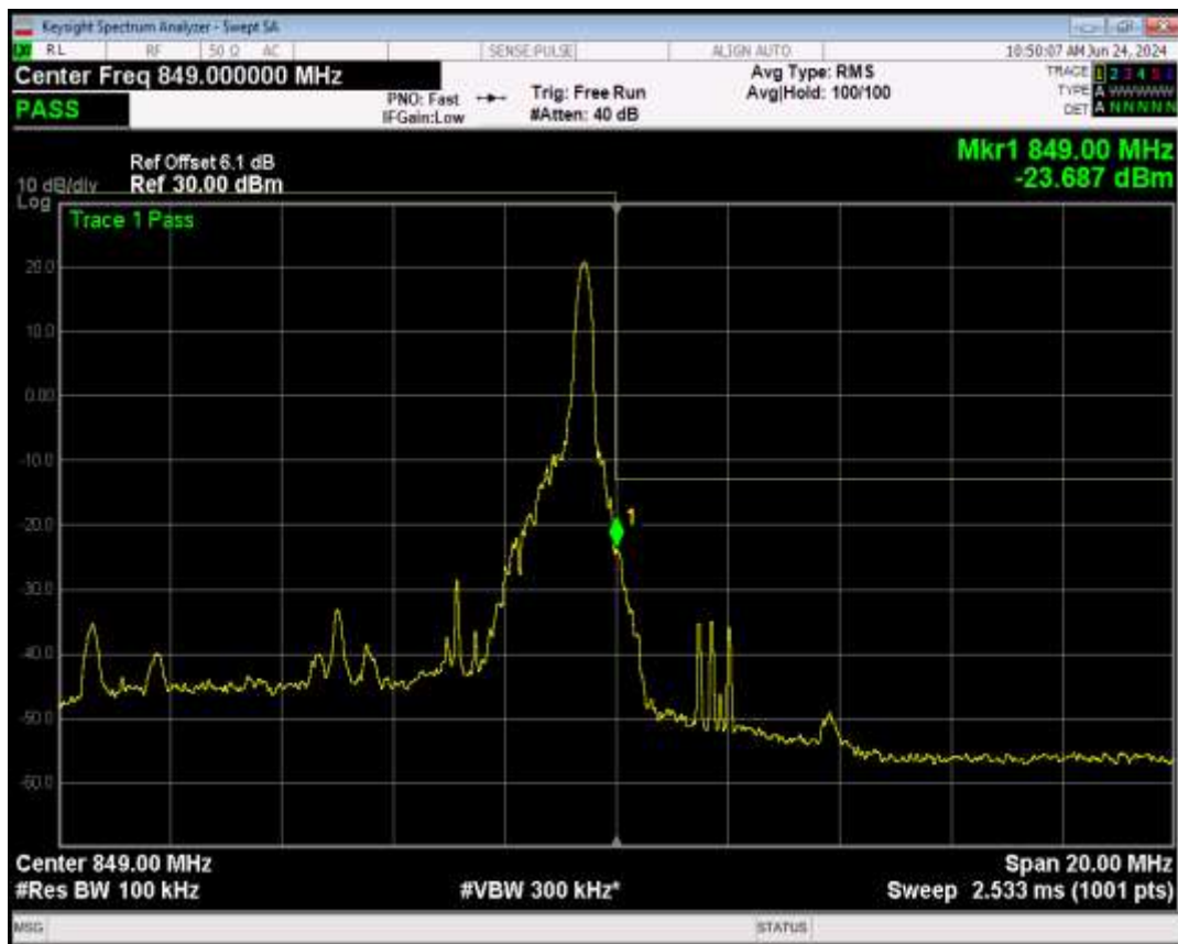
Band5 16QAM BW=10MHz Channel=20600 RB Size=50 Position=#0
