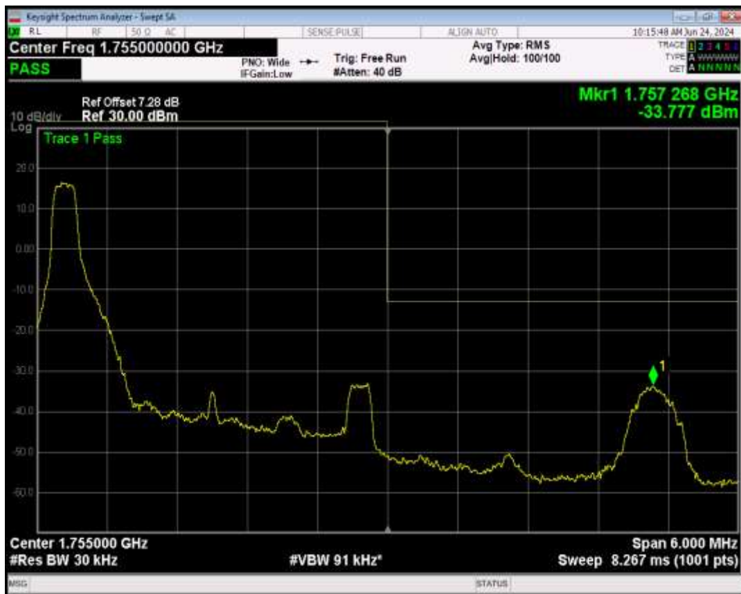
Band4 QPSK BW=3MHz Channel=20385 RB Size=1 Position=#Max
