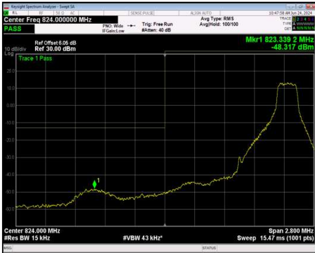
Band5 QPSK BW=1.4MHz Channel=20407 RB Size=6 Position=#0
