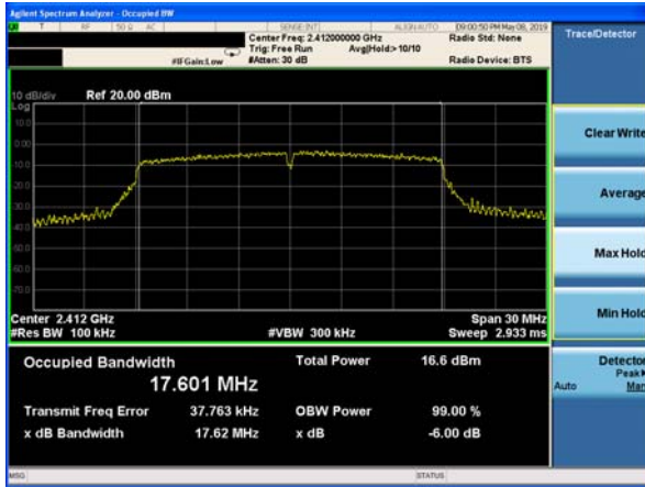
(802.11 N20) 6dB Bandwidth plot on channel 6
