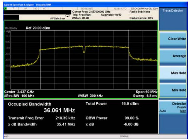
(802.11N40) 6dB Bandwidth plot on channel 11
