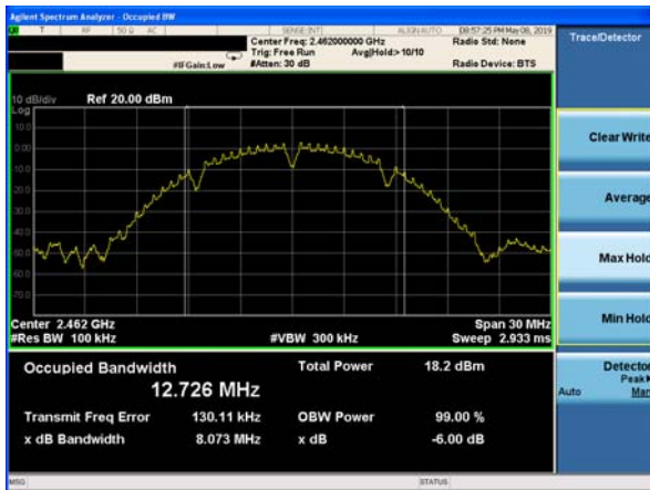
(802.11b) 6dB Bandwidth plot on channel 11
