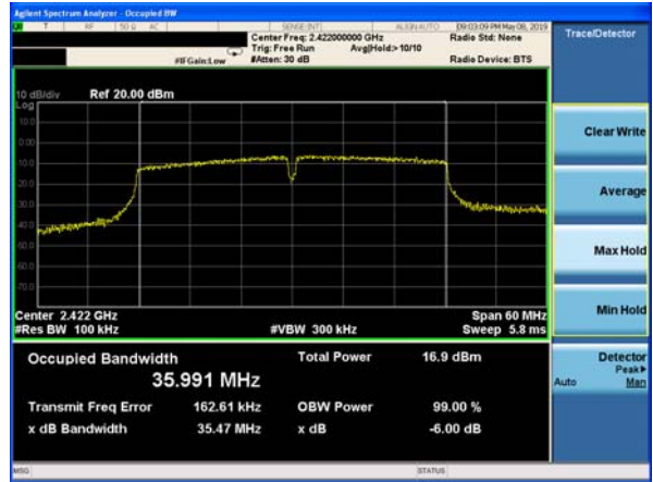
(802.11 N40) 6dB Bandwidth plot on channel 6
