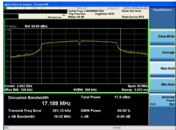
(802.11g) 6dB Bandwidth plot on channel 11
