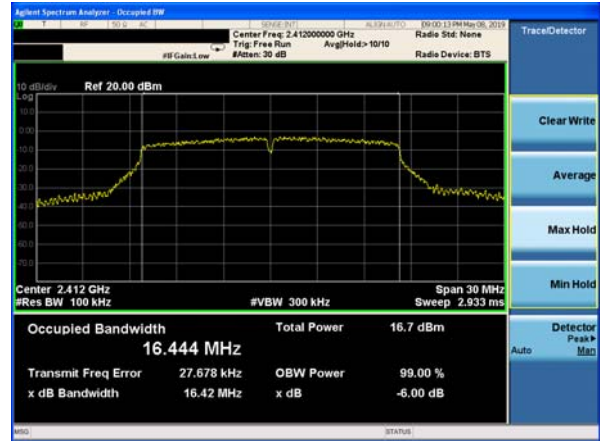
(802.11g) 6dB Bandwidth plot on channel 6
