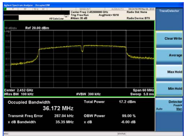
(802.11N40) 6dB Bandwidth plot on channel 11
