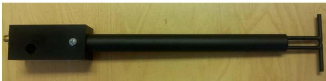
Figure 1 – MVG COMOSAR Validation Dipole
