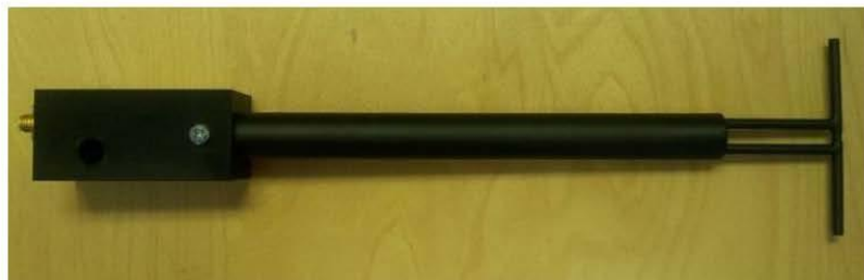
Figure 1 – MVG COMOSAR Validation Dipole
