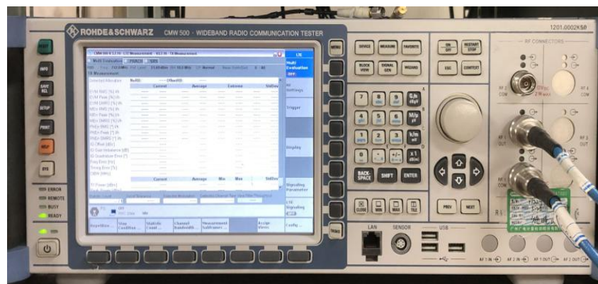
CMW 500 (2G/3G/4G Test Equipment)
