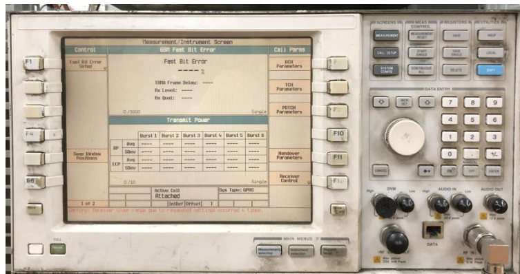
Agilent 8960 (2G/3G Test Equipment)
