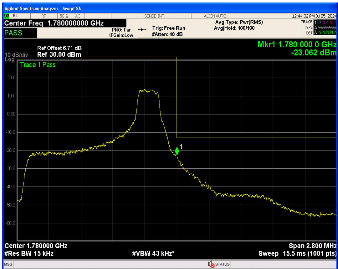
Band66 16QAM BW=1.4MHz Channel=132665 RB Size=6 Position=#0
