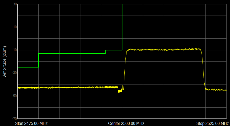
Band7 QPSK BW=20MHz Channel=20850 RB Size=100 Position=#0
