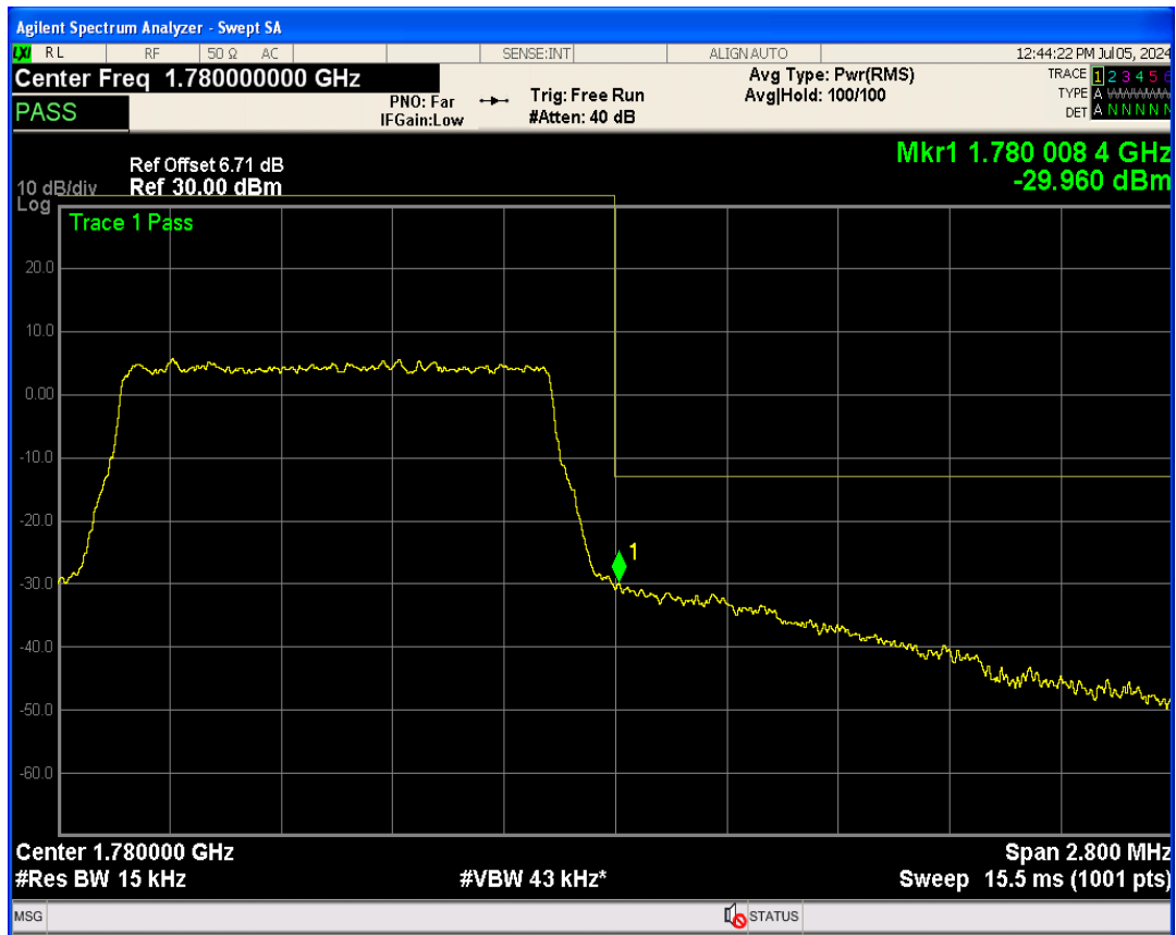
Band66 16QAM BW=1.4MHz Channel=132665 RB Size=1 Position=#Max
