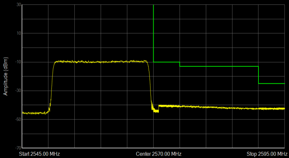
Band7 QPSK BW=20MHz Channel=21350 RB Size=100 Position=#0
