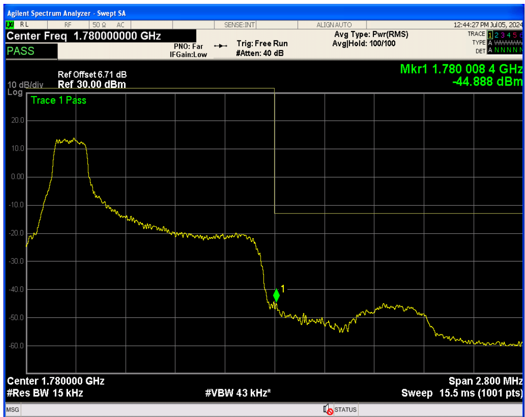
Band66 QPSK BW=1.4MHz Channel=132665 RB Size=6 Position=#0
