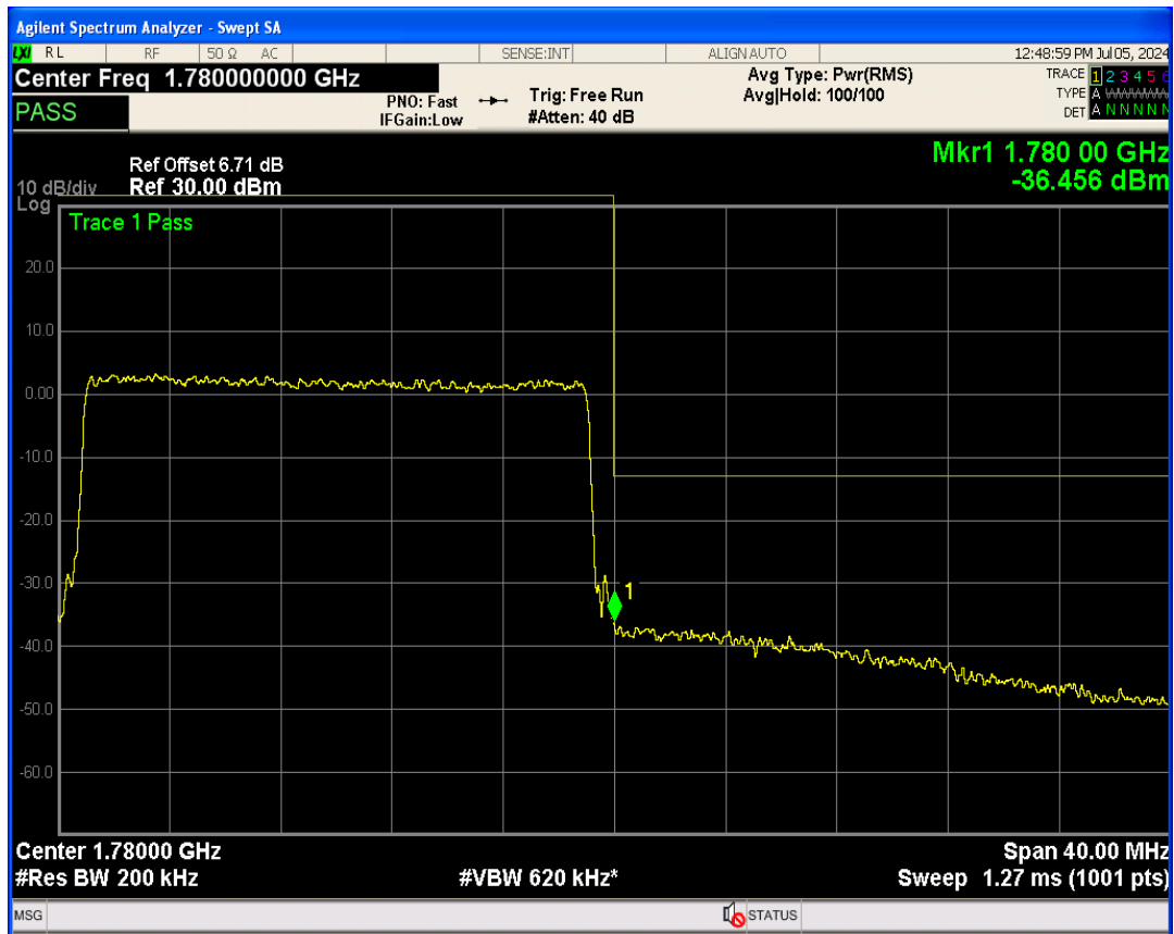
Band7 QPSK BW=5MHz Channel=20775 RB Size=1 Position=#0
