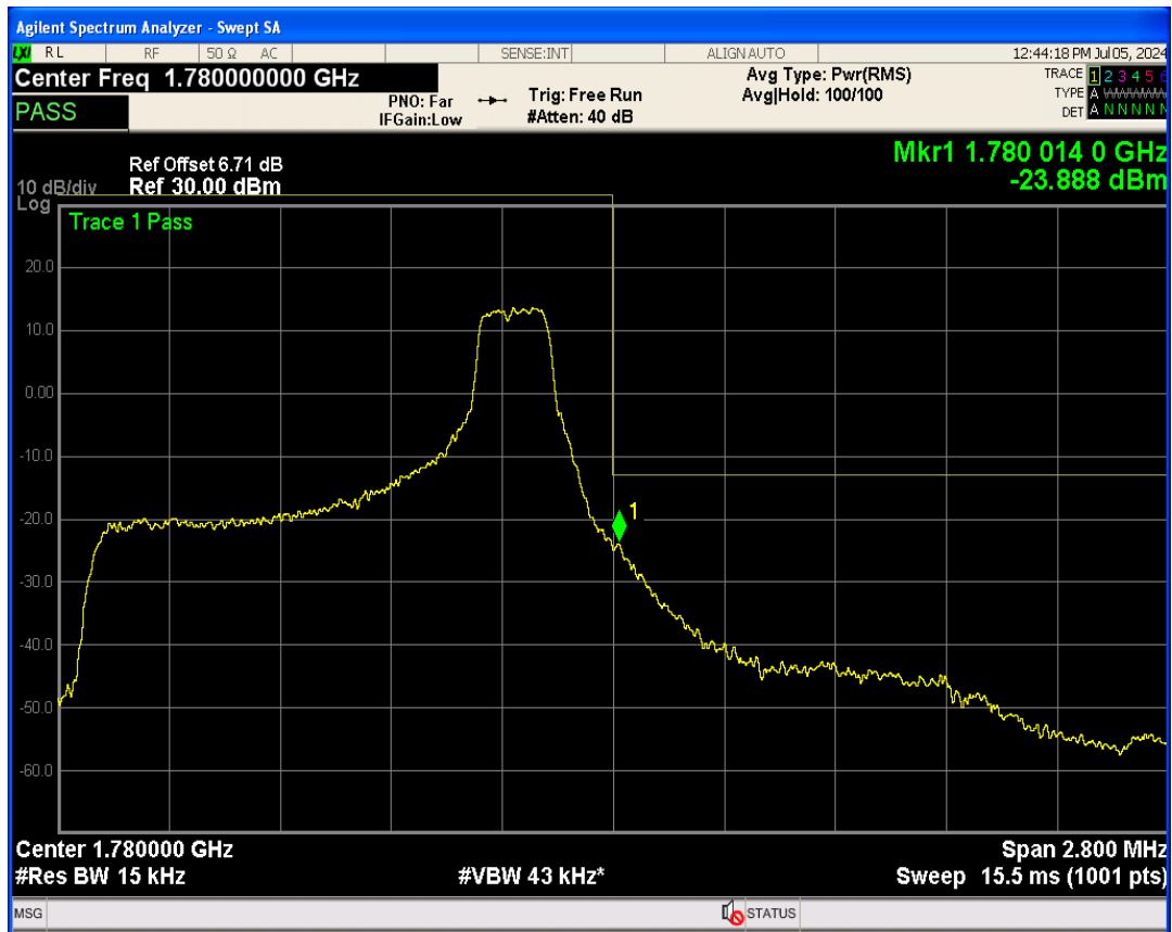
Band66 16QAM BW=1.4MHz Channel=132665 RB Size=1 Position=#0
