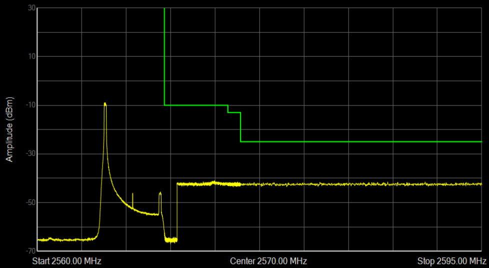
Band7 16QAM BW=5MHz Channel=21425 RB Size=1 Position=#0
