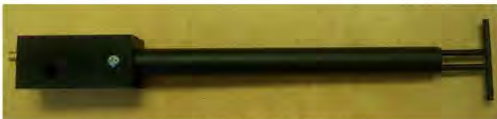
Figure 1 – MVG COMOSAR Validation Dipole
