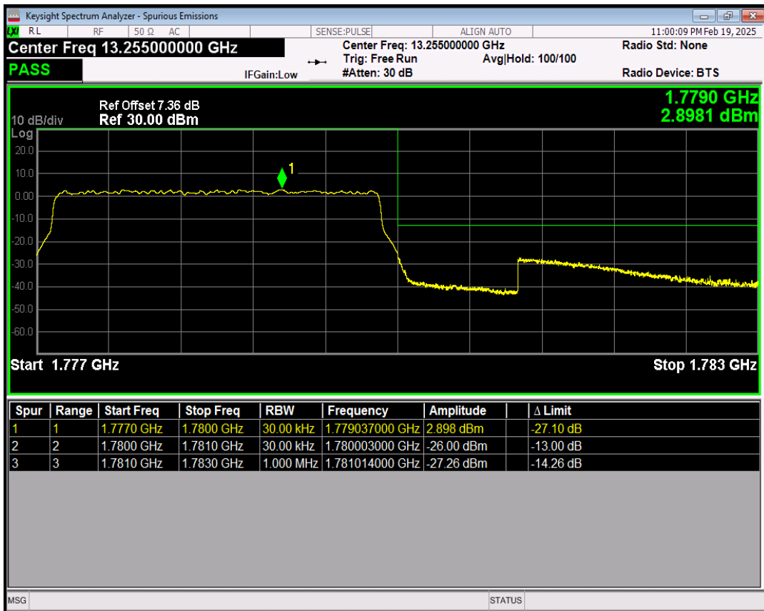
Band66 16QAM BW=3MHz Channel=132657 RB Size=1 Position=#0
