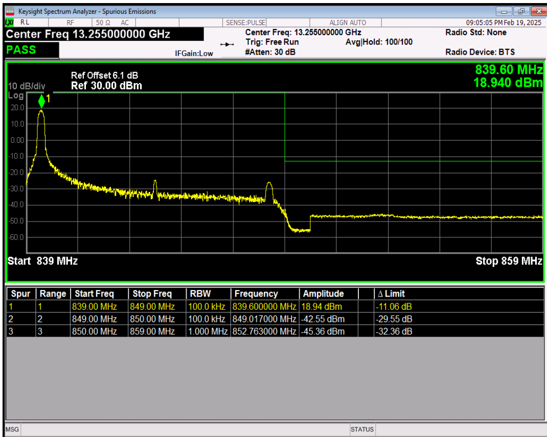
Band5 QPSK BW=10MHz Channel=20600 RB Size=1 Position=#Max
