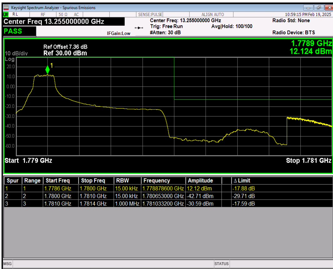
Band66 QPSK BW=1.4MHz Channel=132665 RB Size=1 Position=#Max
