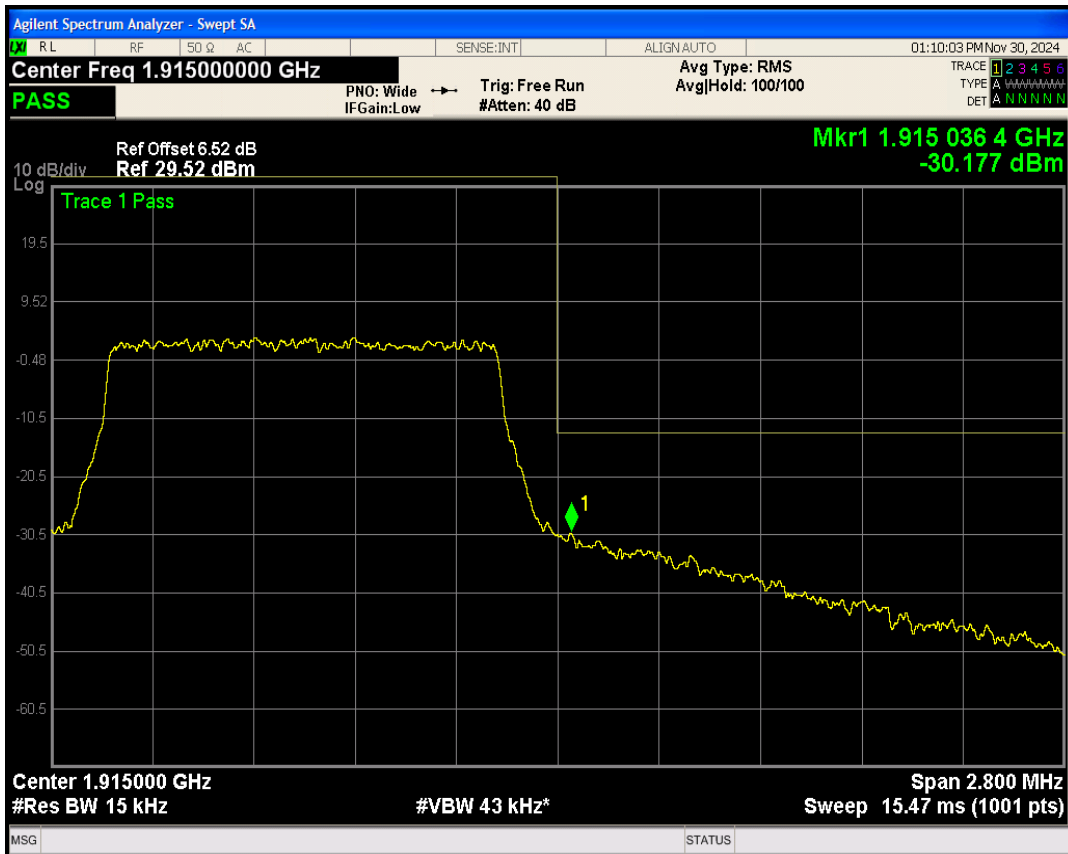
Band25 QPSK BW=3MHz Channel=26055 RB Size=15 Position=#0
