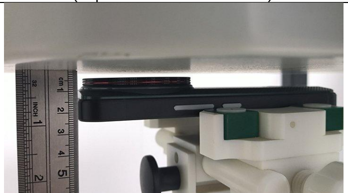
Right Side (Separation distance of 10mm)
