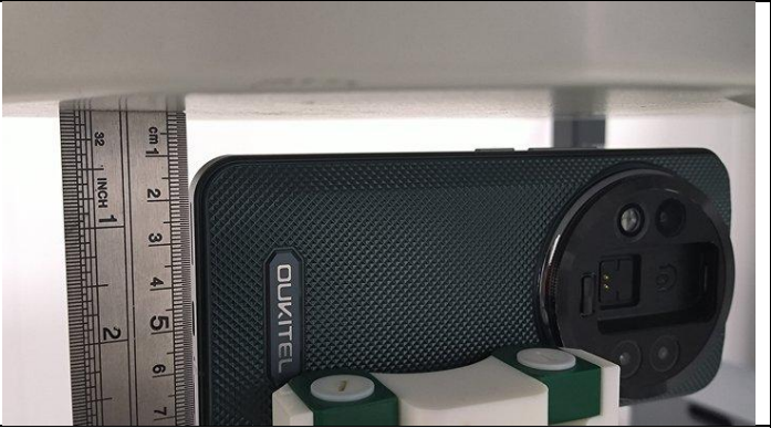
Bottom Side (Separation distance of 10mm)
