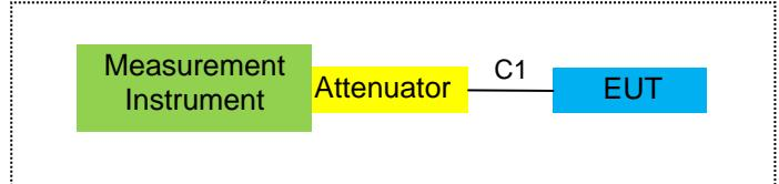
For Peak-to Average Ratio, Occupied Bandwidth, Conducted Band edge and Conducted Spurious Emission
