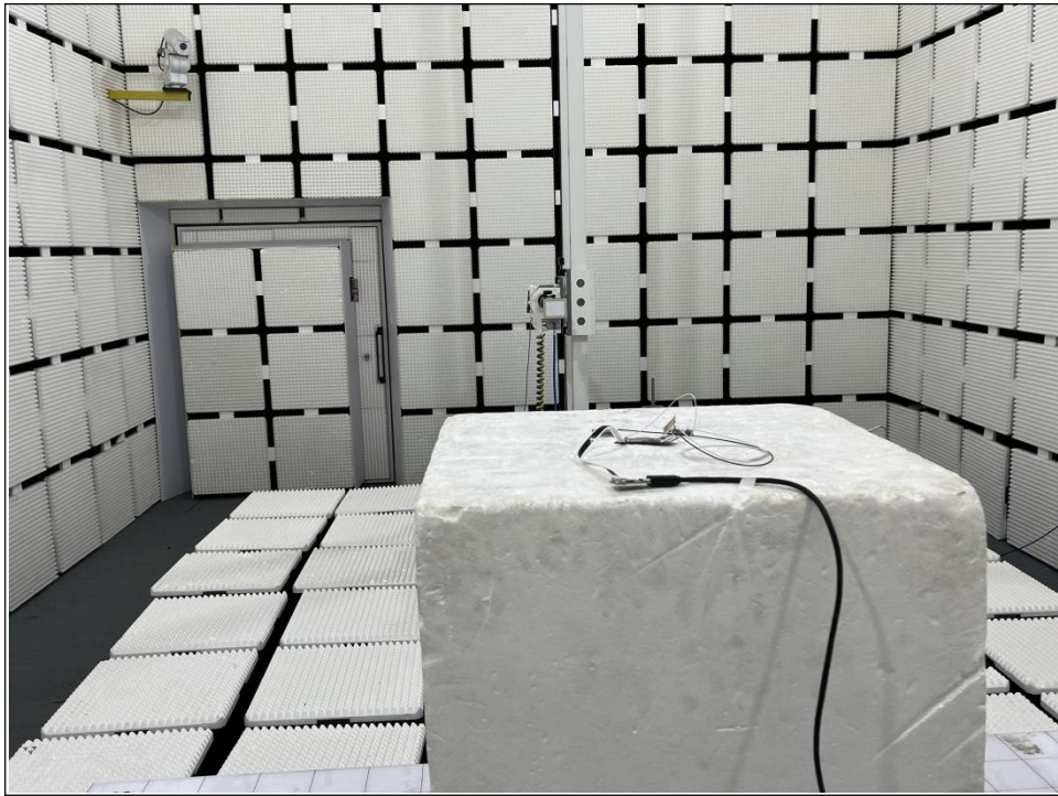
RADIATED EMISSION TEST (18GHz ~ 40GHz)
