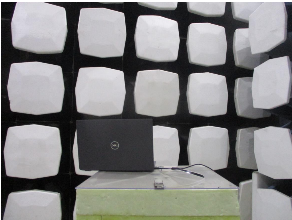
The EUT was placed at the center of turntable
