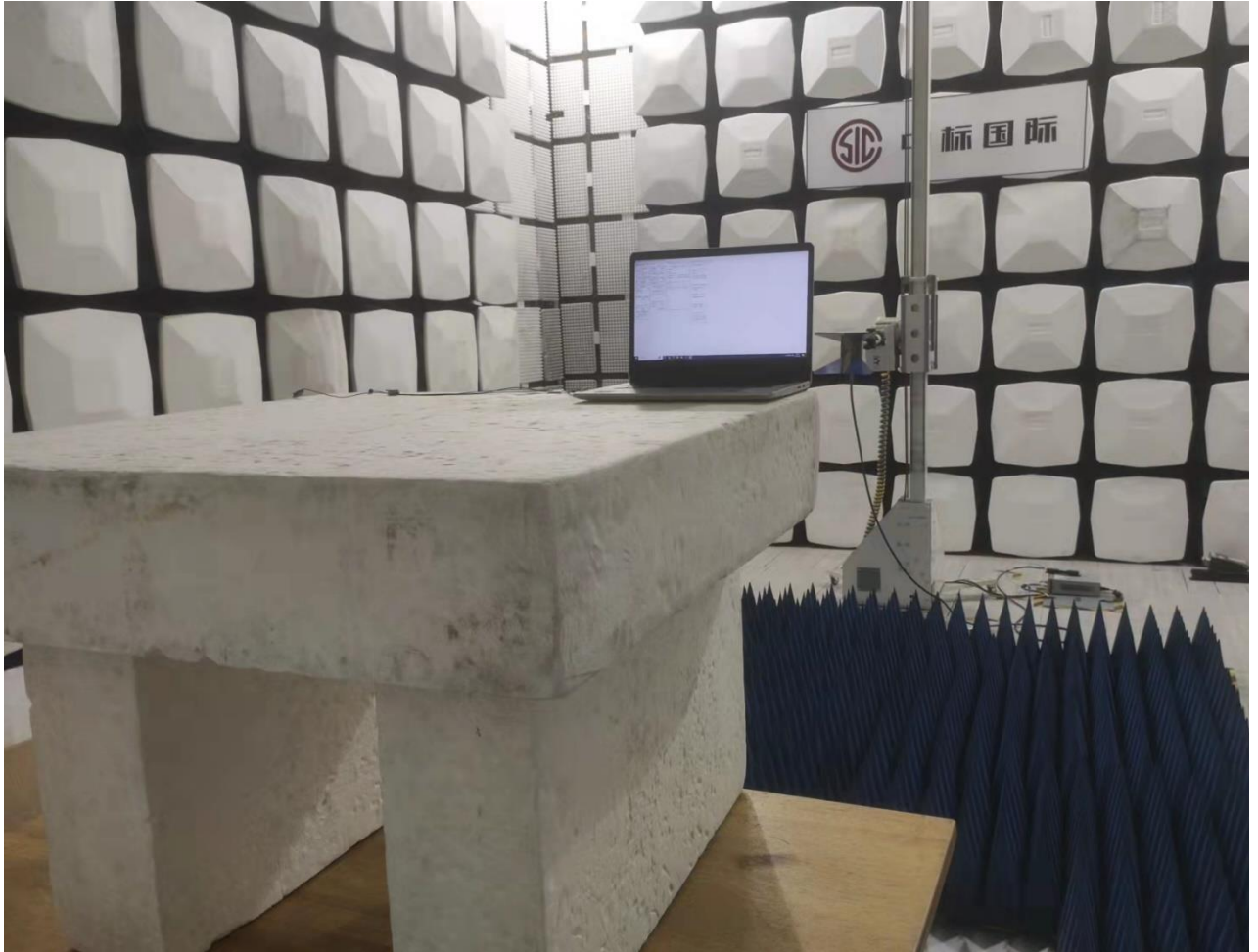
Photograph 2: Set-up for Radiated Spurious Emission, Above 1GHz
