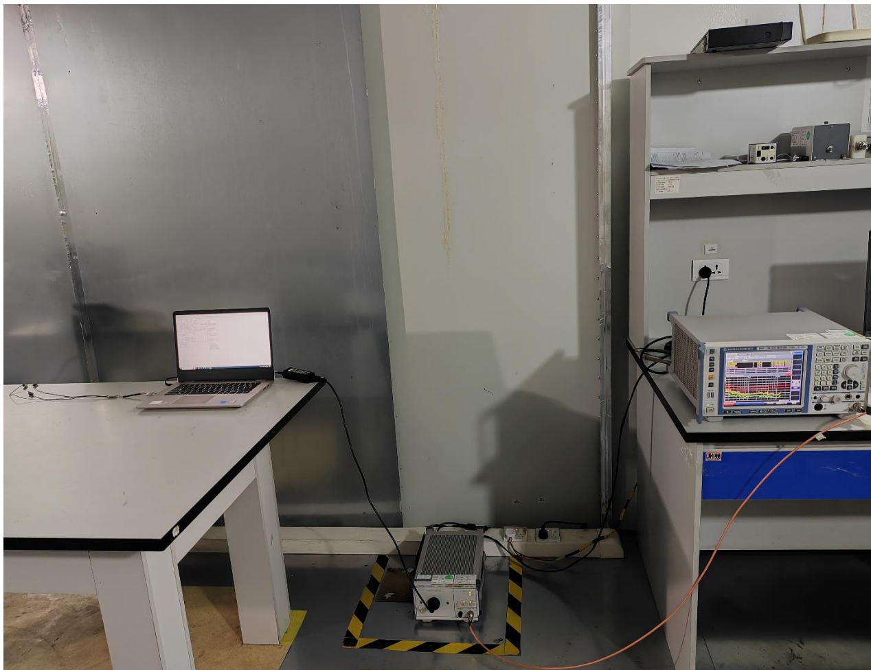
Photograph 3: Set-up for Conducted Emission on AC Mains
