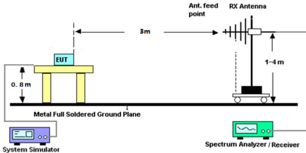
For radiated test from above 1GHz
