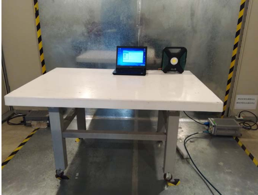
Conducted Emissions (Side View)
