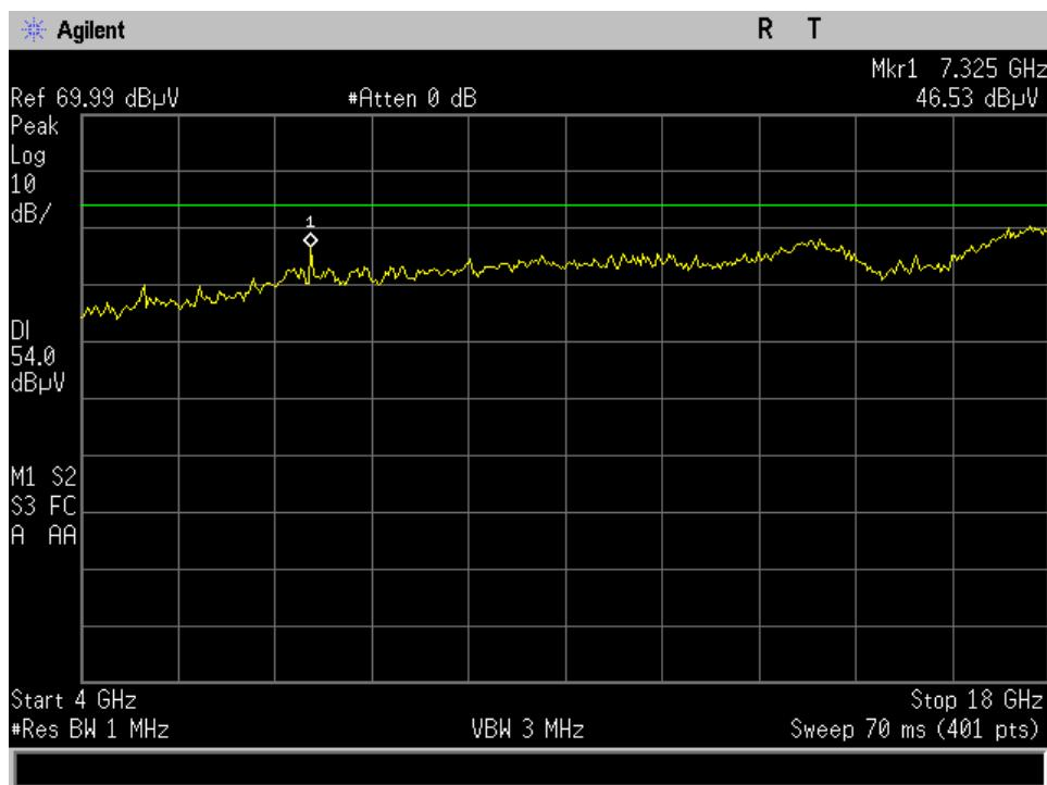
Measurements were taken up to the 10<sup>th</sup> harmonic of the device. No emissions were detected from 18-25 GHz, only noise floor was measured.
