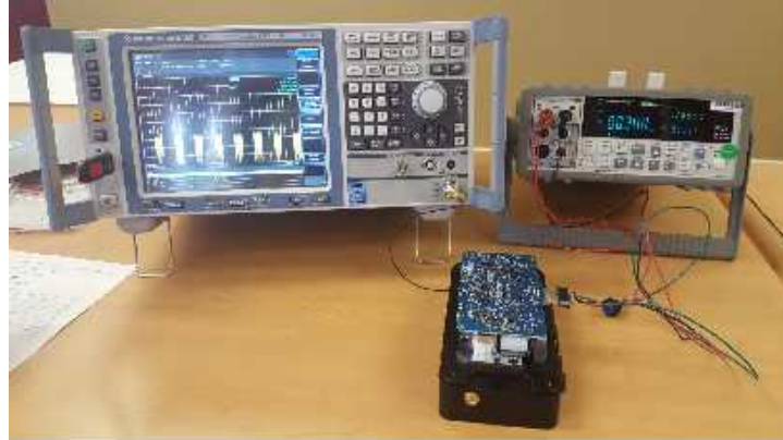
Figure 5: Conducted RF Test Setup Photograph(s).
