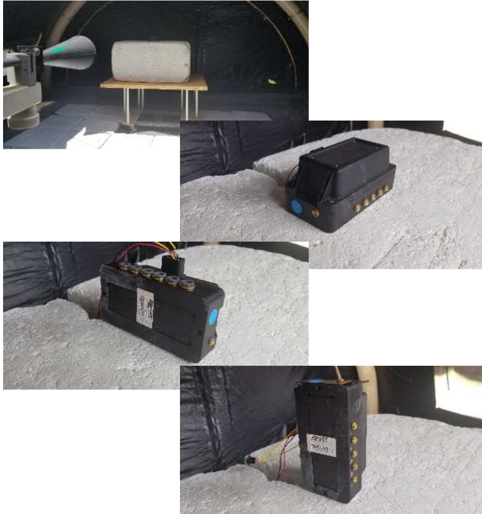
Figure 4: Radiated Emissions Test Setup Photograph(s).
