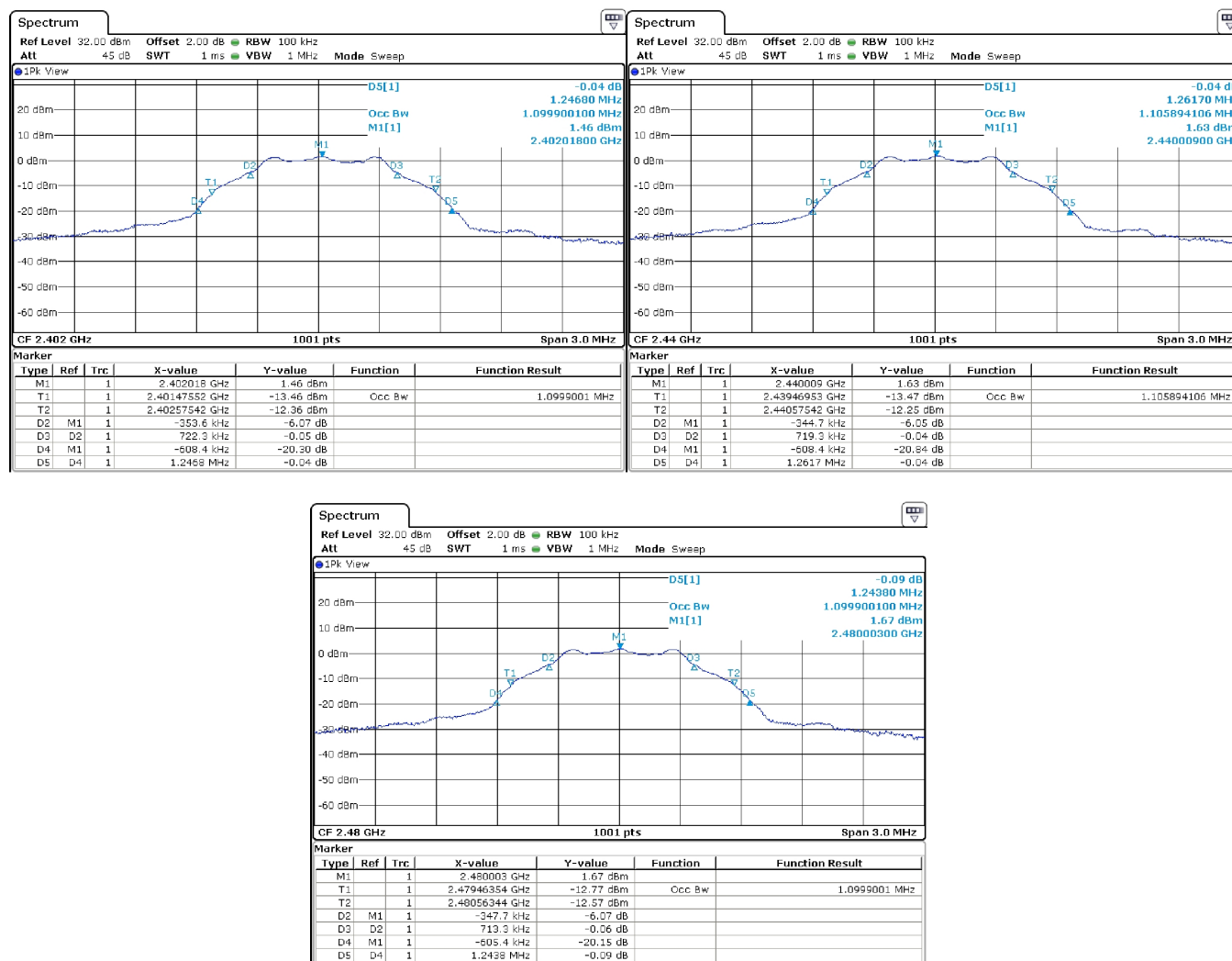
Figure 7: Intentional Emission Bandwidth.
