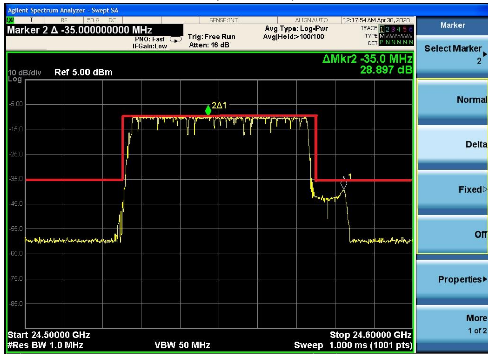
Figure 2 – Modified EchoGuard CR FCC Spectrum Mask 10MHz/div Compliance tested at Echodyne. Shows compliance with first 25dB mask step required by FCC. All other offsets unchanged.
