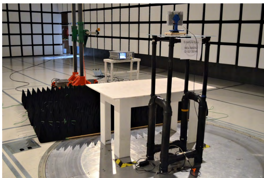
Figure 3.6-6: Radiated Emissions Test Setup – 18-40 GHz (Back)
