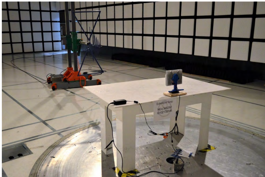
Figure 3.6-2: Radiated Emissions Test Setup – below 1GHz (Back)
