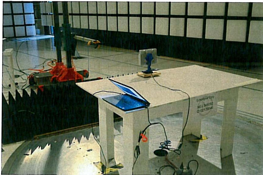
Figure 3.6-10: Radiated Emissions Test Setup – 75-110 GHz (Back)
