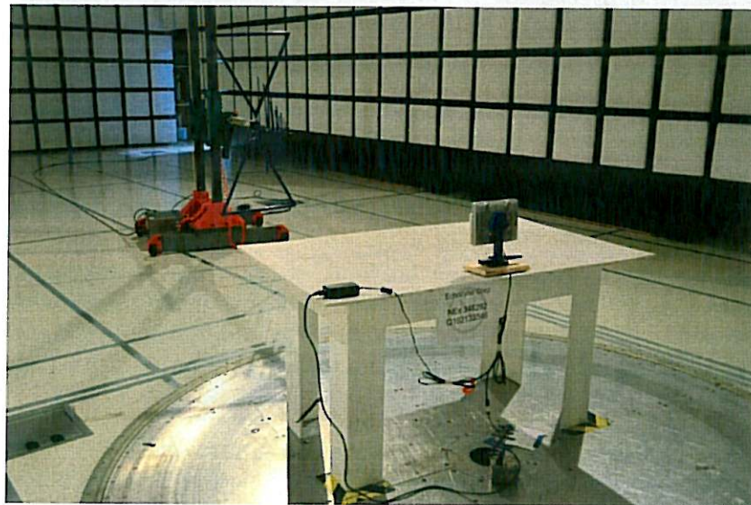
Figure 3.6-2: Radiated Emissions Test Setup – below 1GHz (Back)
