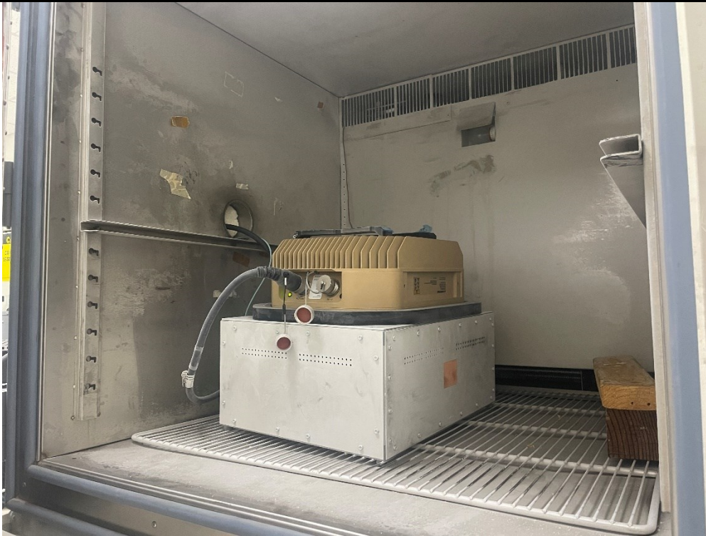
Figure 18 – Frequency stability test setup
