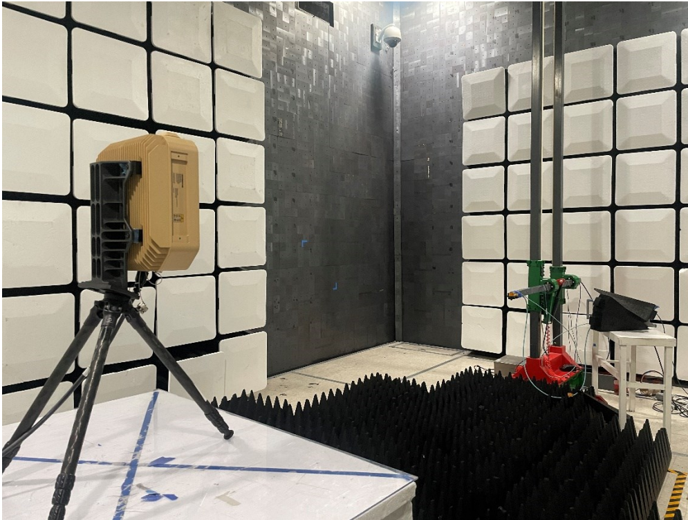
Figure 15 - Radiated emissions above 1 GHz (50 – 75 GHz), rear view.
