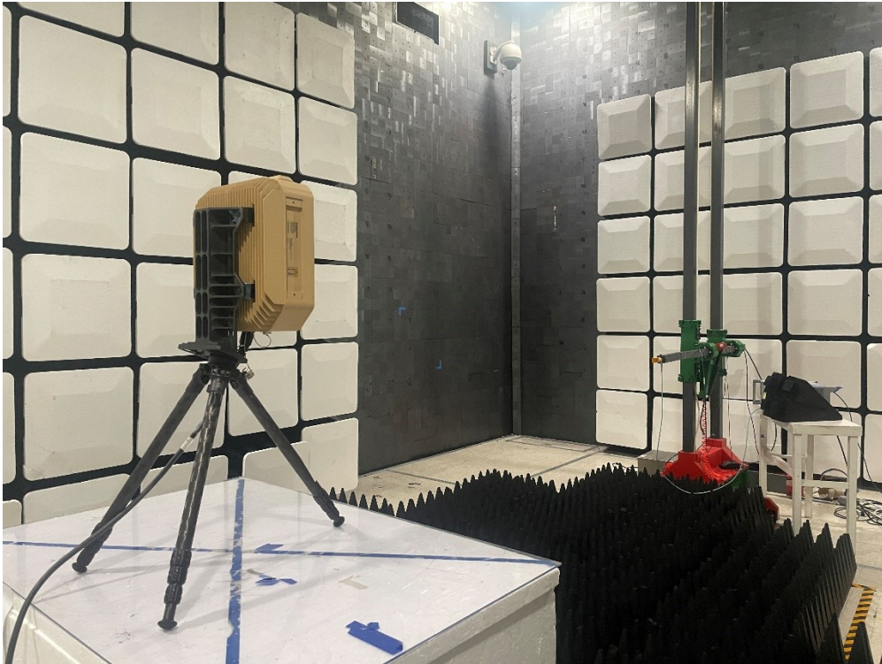
Figure 13 - Radiated emissions above 1 GHz (40 – 50 GHz), rear view.
