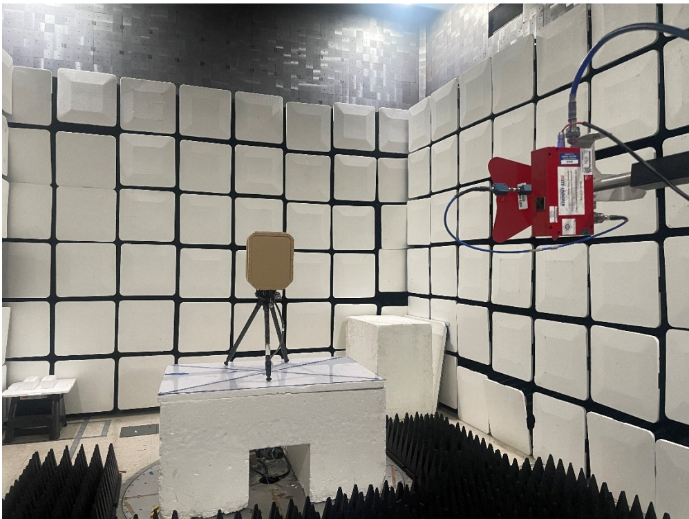
Figure 6 - Radiated emissions above 1 GHz (1– 18 GHz), front view.
