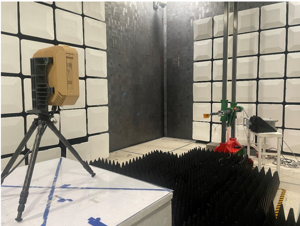
Figure 10 - Radiated emissions above 1 GHz (26.5 – 40 GHz), front view.
