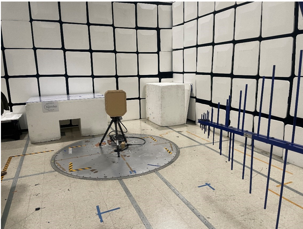
Figure 4 - Radiated emissions below 1 GHz (0.03 – 1 GHz), front view.
