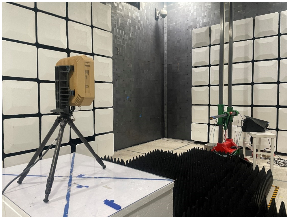
Figure 17 - Radiated emissions above 1 GHz (75 – 100 GHz), rear view.
