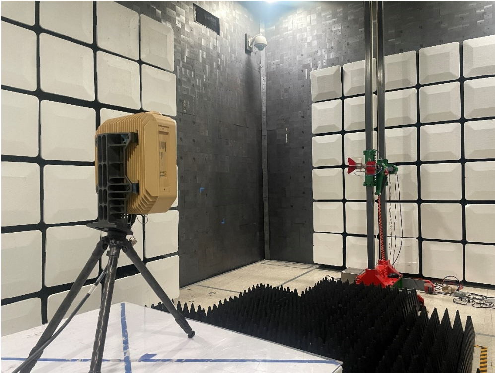
Figure 7 - Radiated emissions above 1 GHz (1 – 18 GHz), rear view.
