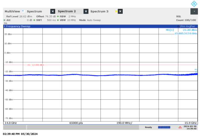
Figure 8.4-70: Emission mask, beyond \pm 250\% of BW (low frequency range), High channel: 16.40 GHz, shortest pulse. (200 MHz BW)
