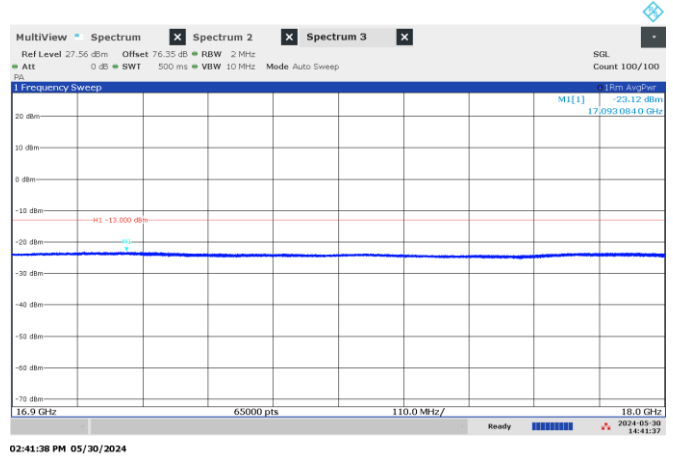
Figure 8.4-72: Emission mask, beyond \pm 250\% of BW (high frequency range), High channel: 16.40 GHz, shortest pulse. (200 MHz BW)
