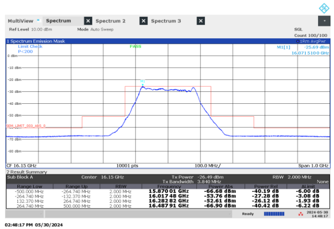
Figure 8.4-68: Emission mask, Middle channel: 16.15 GHz, shortest pulse. (200 MHz BW)
