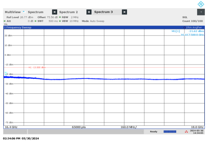
Figure 8.4-66: Emission mask, beyond \pm 250\% of BW (high frequency range), Low channel: 15.90 GHz, shortest pulse. (200 MHz BW)
