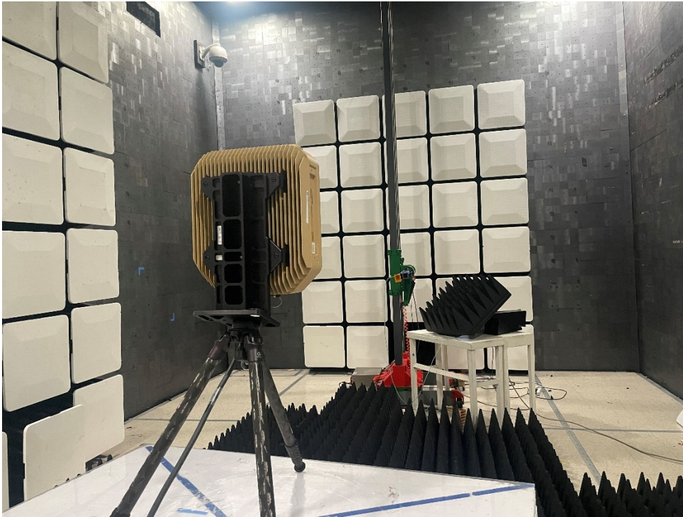
Figure 11 - Radiated emissions above 1 GHz (26.5 – 40 GHz), rear view.
