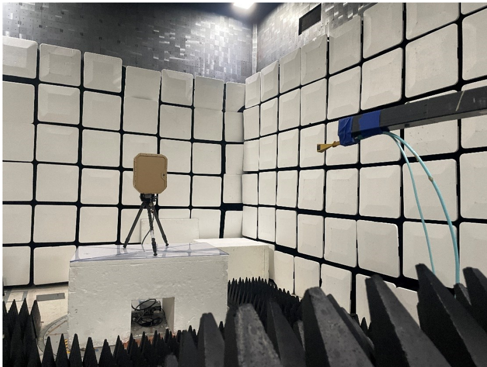
Figure 16 - Radiated emissions above 1 GHz (75 – 100 GHz), front view.
