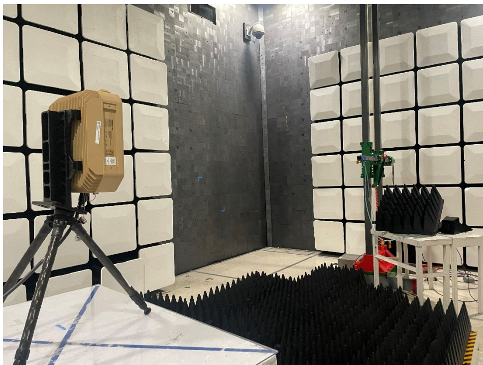
Figure 17 - Radiated emissions above 1 GHz (75 – 100 GHz), rear view.
