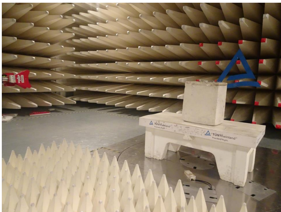
Test setup Frequency Range 18GHz-26.5GHz Double ridged wave guide Horn Antenna
