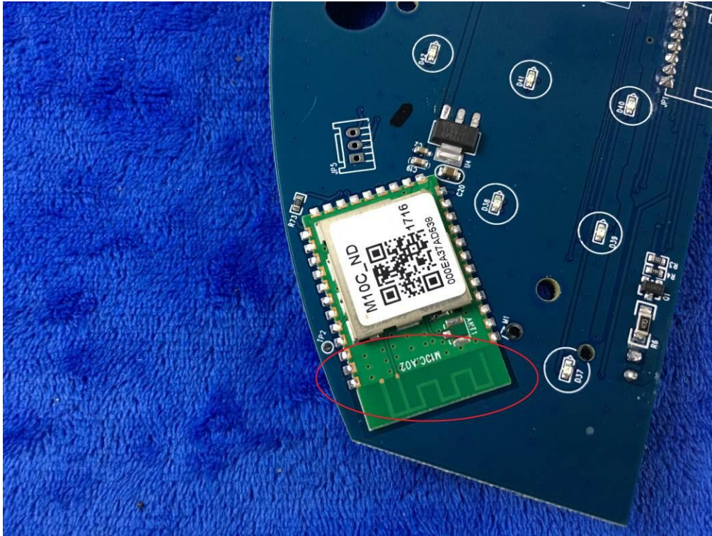
WIFI - Antenna View
