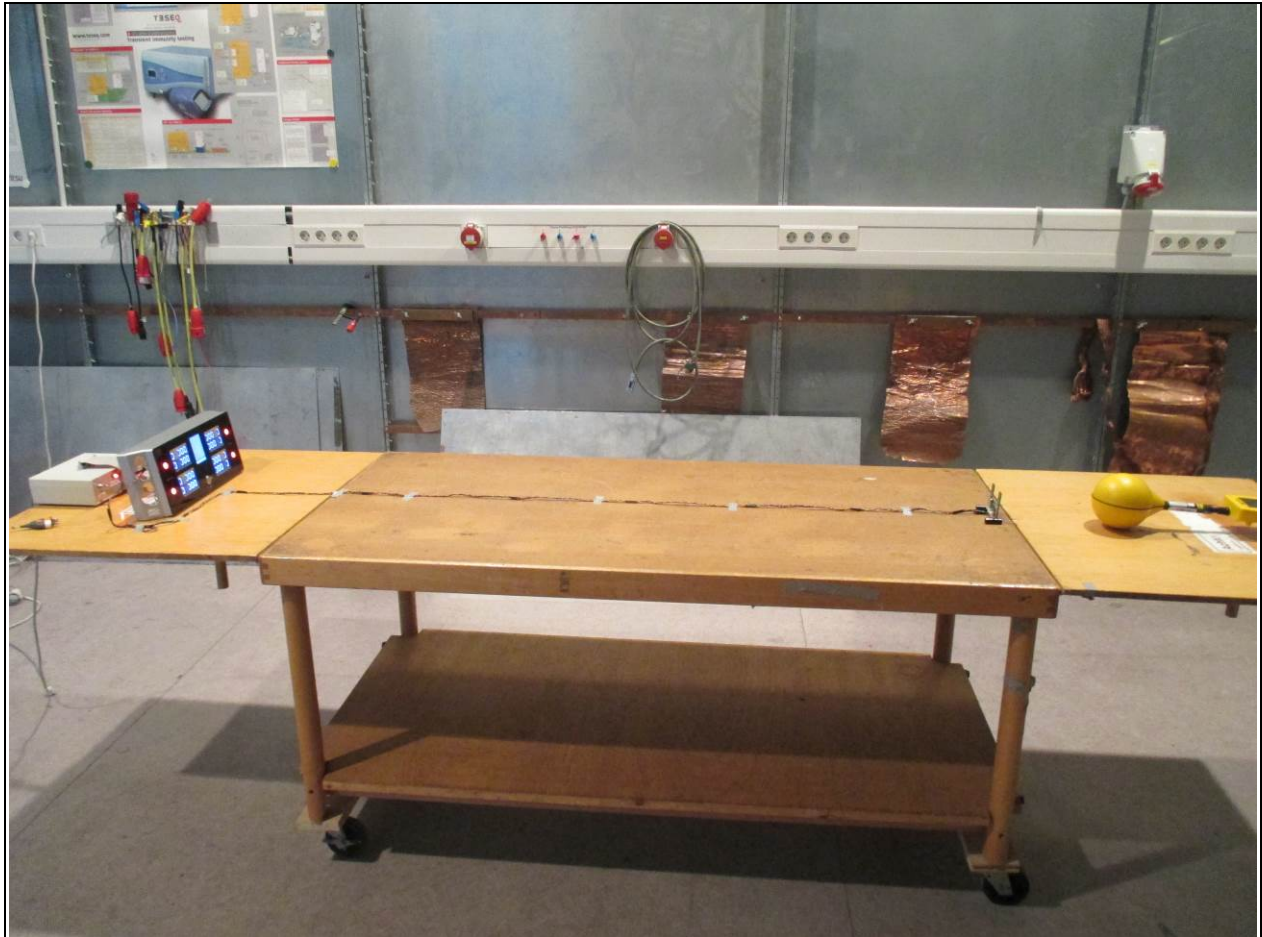
Figure 6-1: General test setup for H/B-field (radiated)
