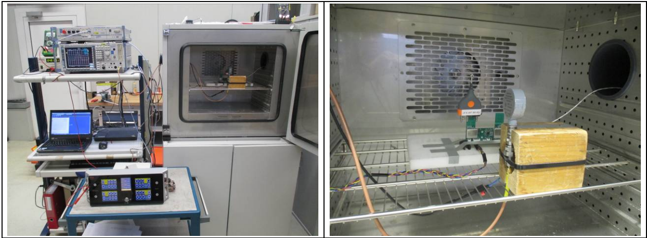
Figure 7-40: Test Setup Occupied Bandwidth – Configuration 5
