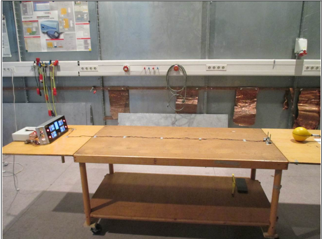
Figure 6-1: General test setup for H/B-field (radiated)
