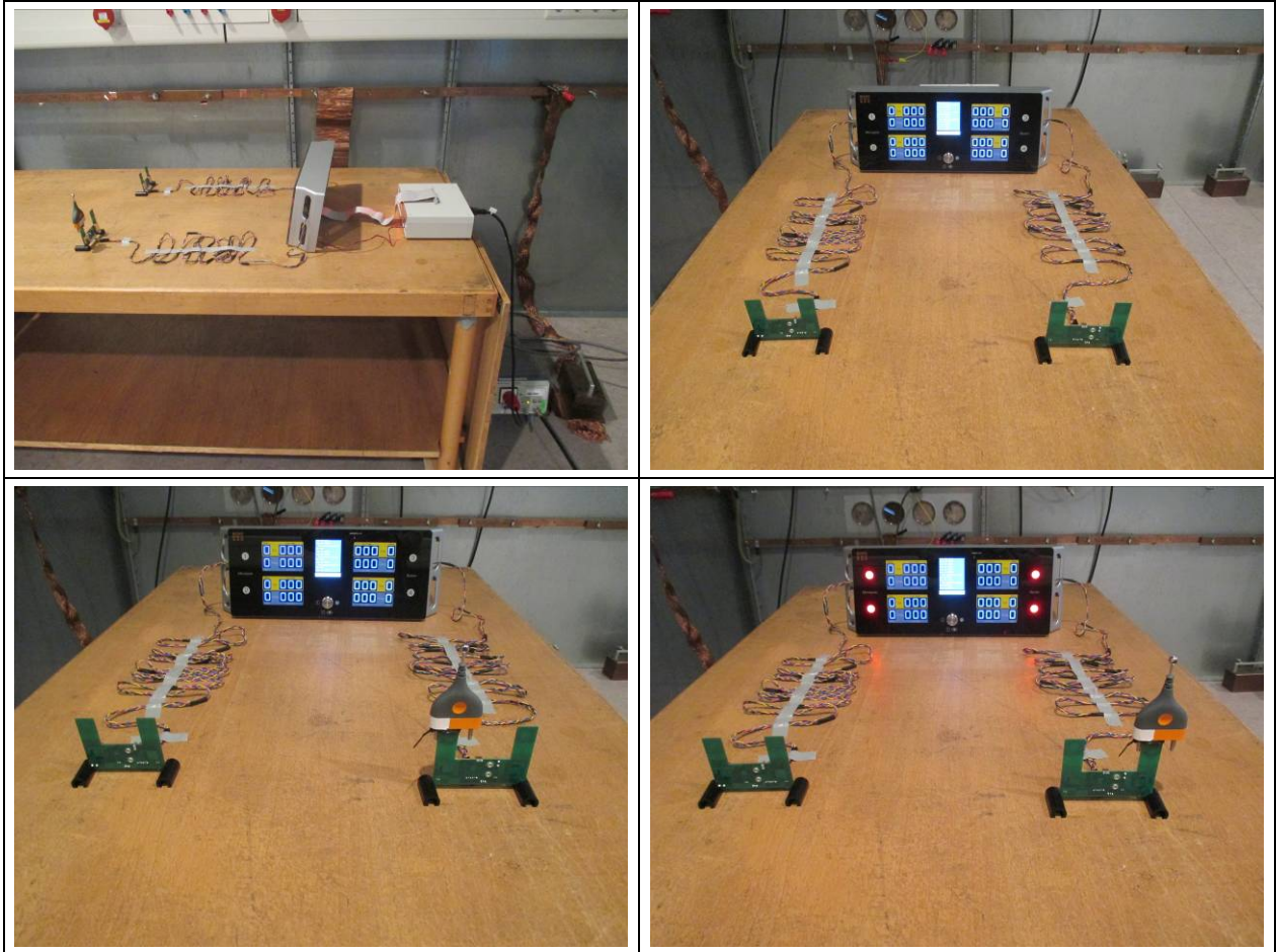
Figure 7-40: Test Setup Conducted Emissions (150 kHz – 30 MHz) – Configurations 11
