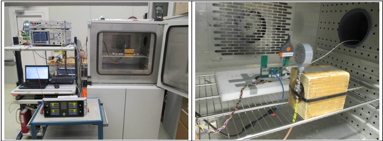
Figure 7-41: Test Setup Occupied Bandwidth – Configuration 5
