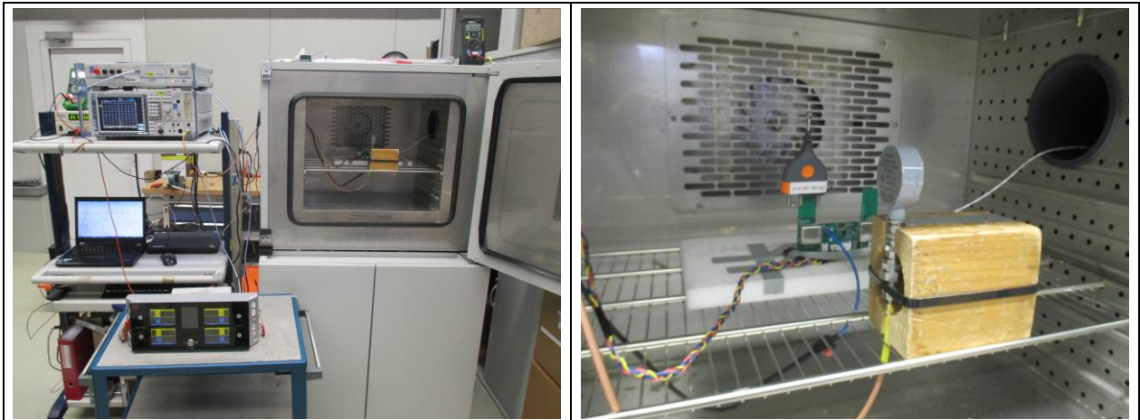
Figure 7-42: Test Setup Occupied Bandwidth – Configuration 6
