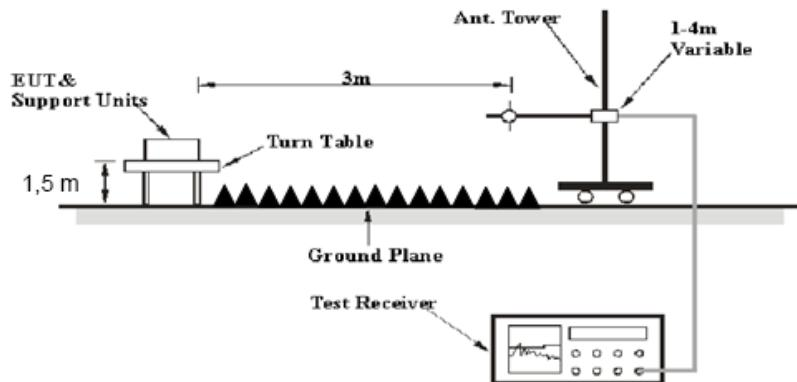
The radiated emission tests were performed in the 3 meters chamber test site A for the range 30MHz to 1GHz and the 3 meters chamber A test site for above 1GHz, using the setup accordance with the ANSI C63.10-2013. The specification used was the FCC 15.209, and FCC 15.247 limits.
