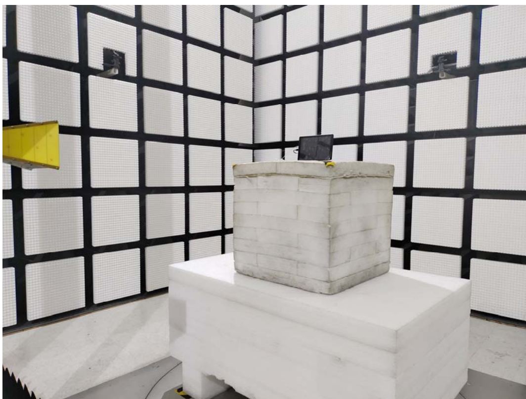
Radiated Emission Above 1GHz View
