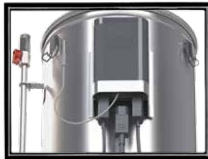
3. Attach all plugs and temperature probe connection. Plug the cord from the pump into the pump inlet underneath the control box, do the same for the plug coming from the boiler. The plug exiting the pump is the pump plug, the plug exiting the boiler base is the heating element plug.
