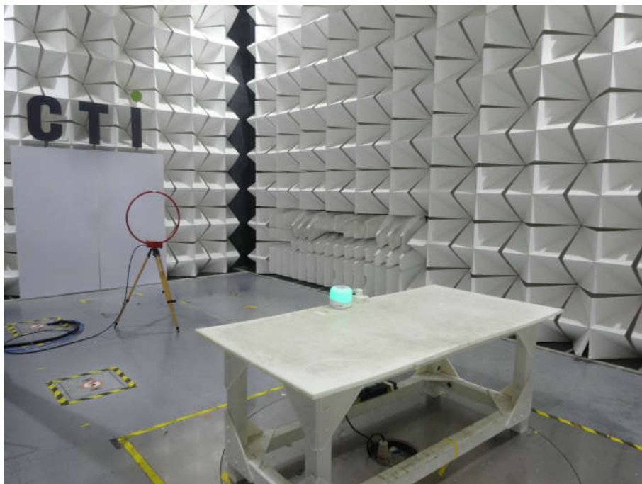
Radiated spurious emission Test Setup-1(9KHz-30MHz)
