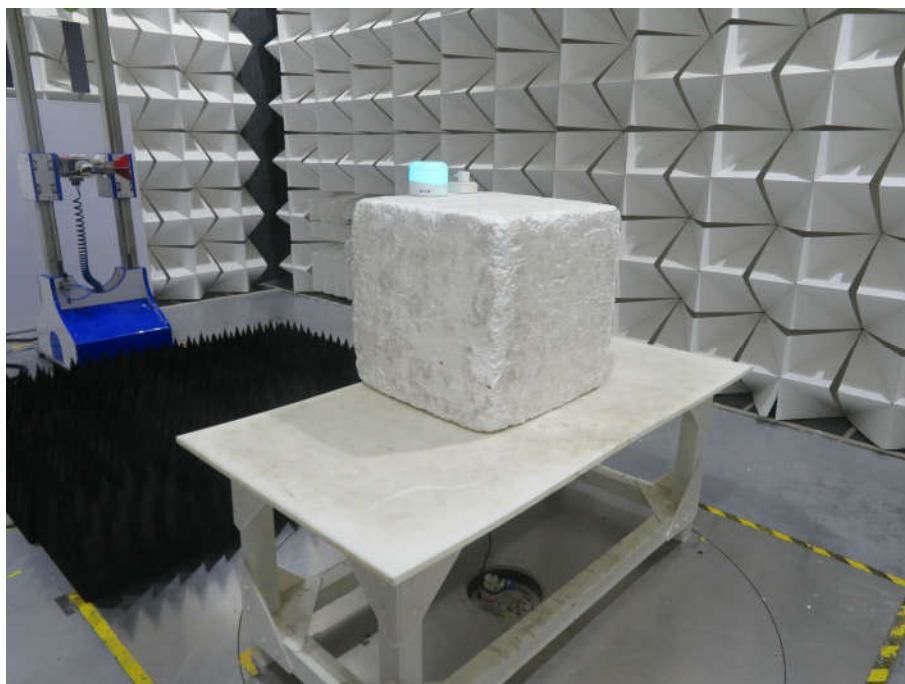
Radiated spurious emission Test Setup-3(Above 1GHz)
