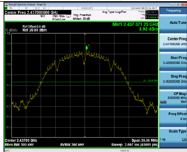
Conducted Emission,Reference Level : 802.11b,2437MHz,1
