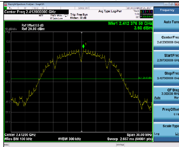
Conducted Emission,1MHz~2300 : 802.11b,2412MHz,1
