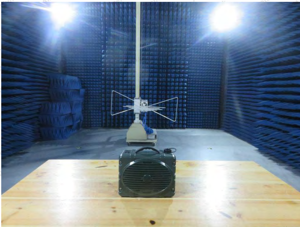
Photo of Radiation Emission Test
