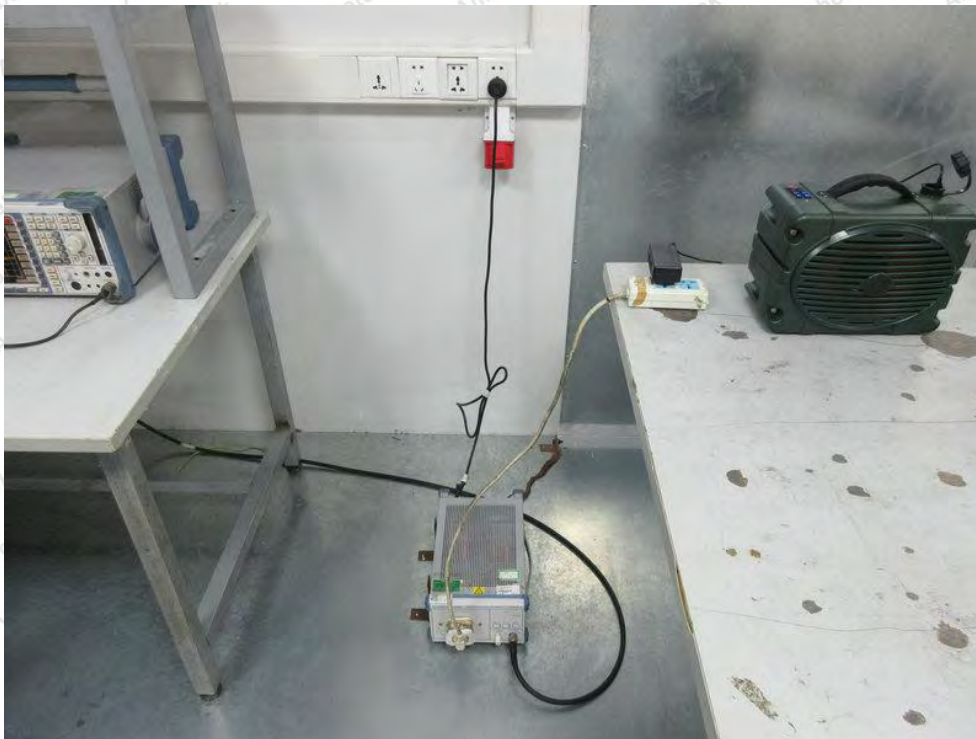
Photo of Conducted Emission Measurement
