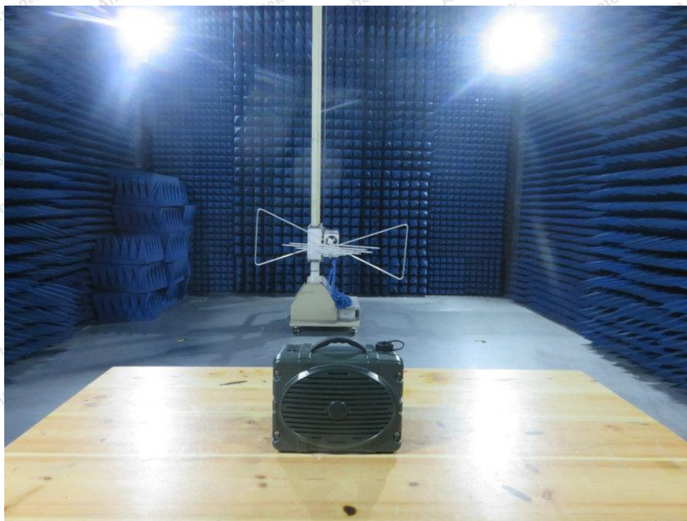
Photo of Radiation Emission Test
