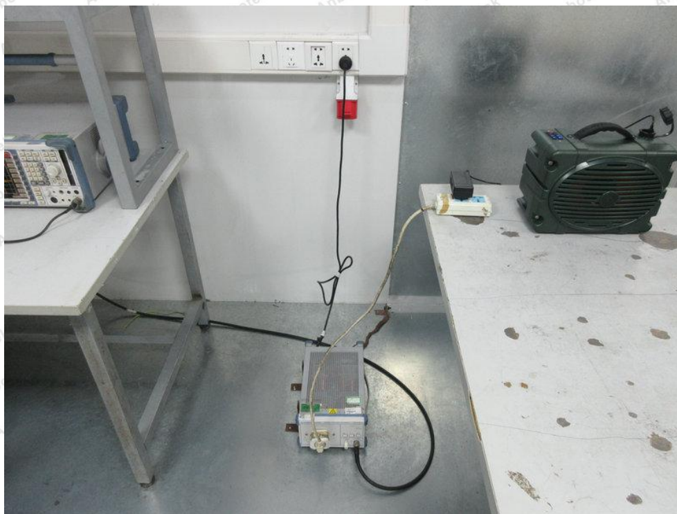
Photo of Conducted Emission Measurement
